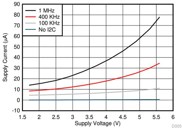
**Figure 8-7. Supply Current vs. I<sup>2</sup>C Bus Clock and Supply Voltage in Shutdown Mode**
