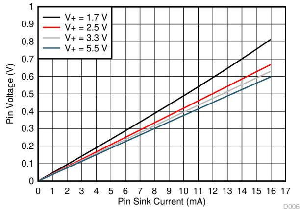
**Figure 8-8. ALERT Pin Output Voltage vs. Sink Current**
