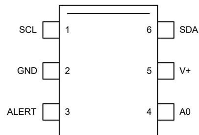
1. Pin 1 is determined by orienting the package marking as indicated in the diagram.
