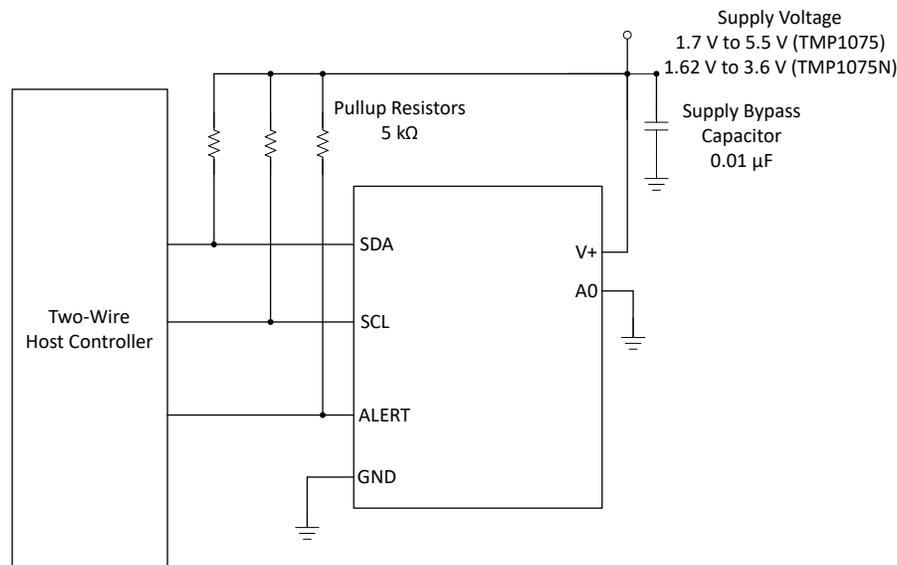
Figure 10-1. Typical Connections
