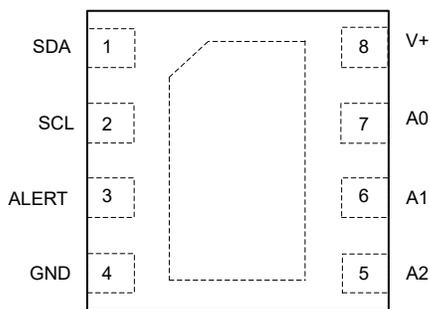
**Figure 7-3. DSG Package 8-Pin WSON Top View**
