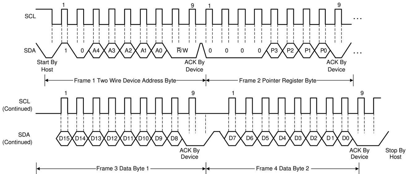
**Figure 9-3. Two-Wire Timing Diagram for Write Word Format**
