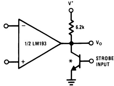
\* OR LOGIC GATE WITHOUT PULL-UP RESISTOR
