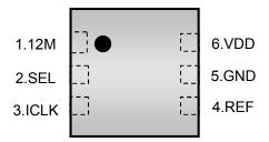
Package: 6-Pin USON (Top View) \*lead-free
