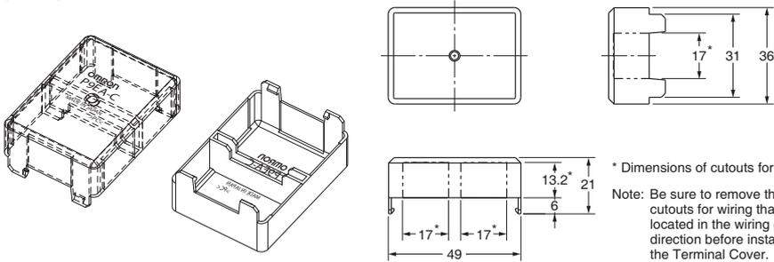
\* Dimensions of cutouts for wiring.
