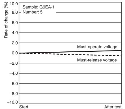
Characteristics were measured after applying a shock of 490 m/s² to the test piece 3 times each in 6 directions along 3 axes. The percentage rate of change is the average value for all of the samples.
