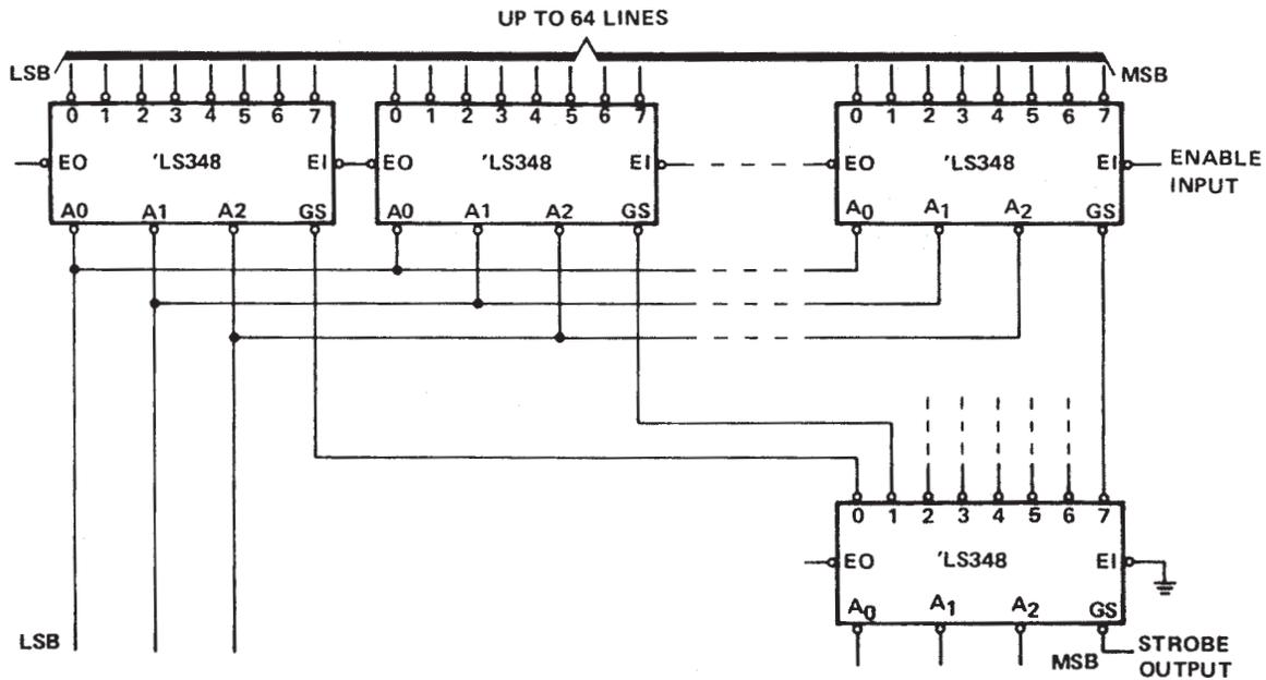
FIGURE 1—PRIORITY ENCODER WITH UP TO 64 INPUTS.
