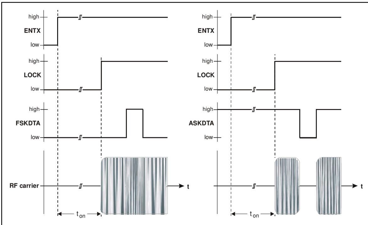
Fig. 5: Timing diagrams for FSK and ASK modulation
