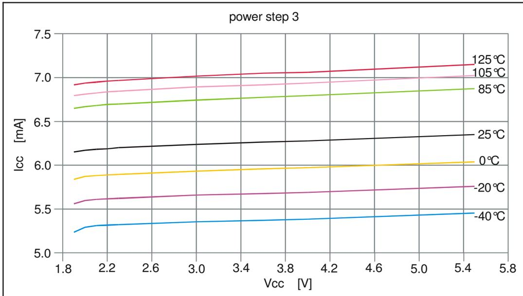
Fig. 10: Supply current in power step 3
