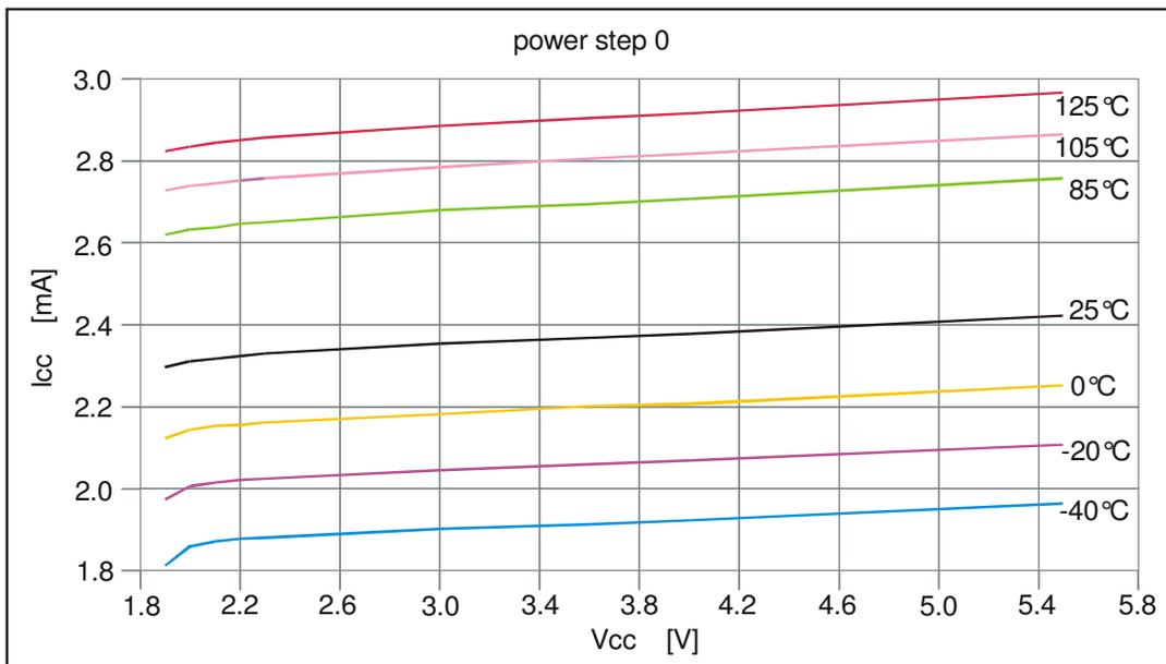
Fig. 7: Supply current in power step 0
