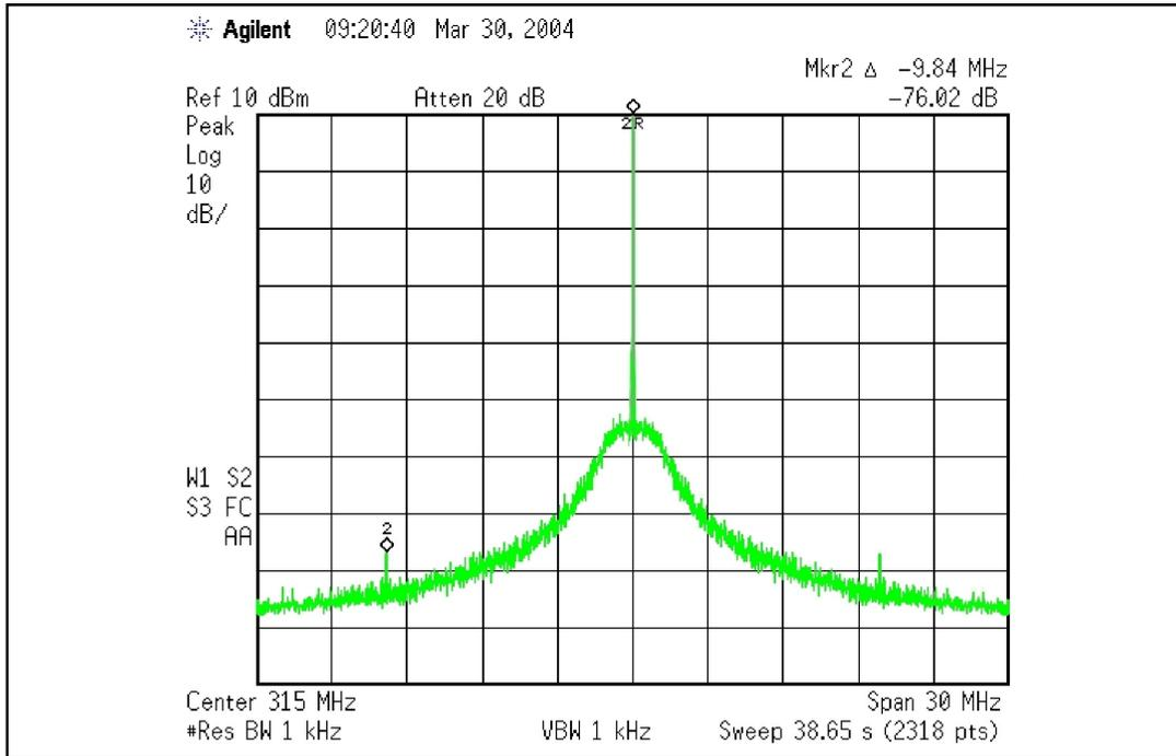
Fig. 16: RF output signal with PLL reference spurs
