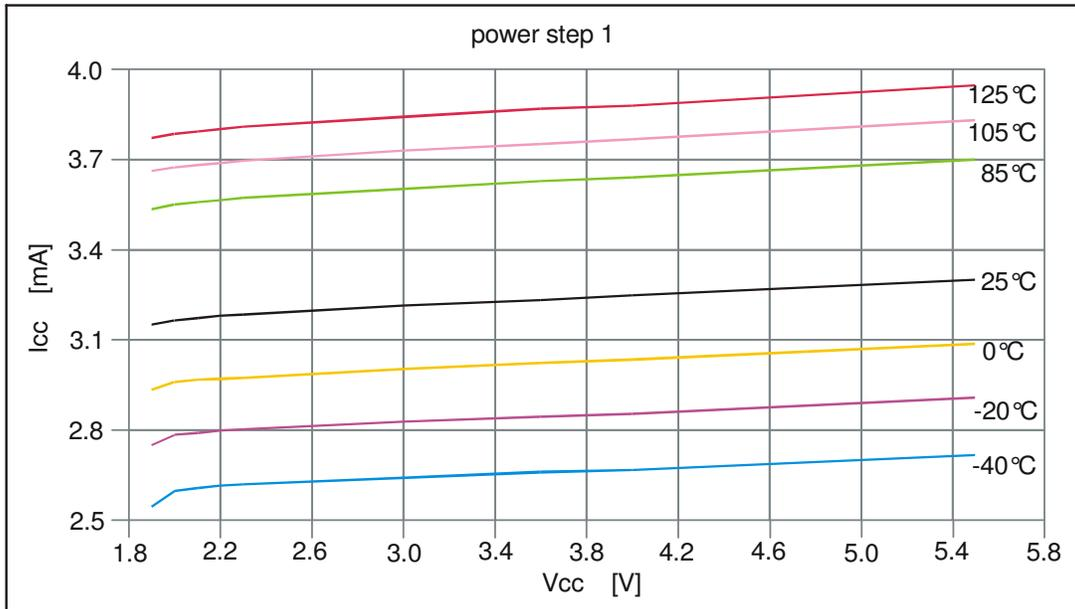
Fig. 8: Supply current in power step 1
