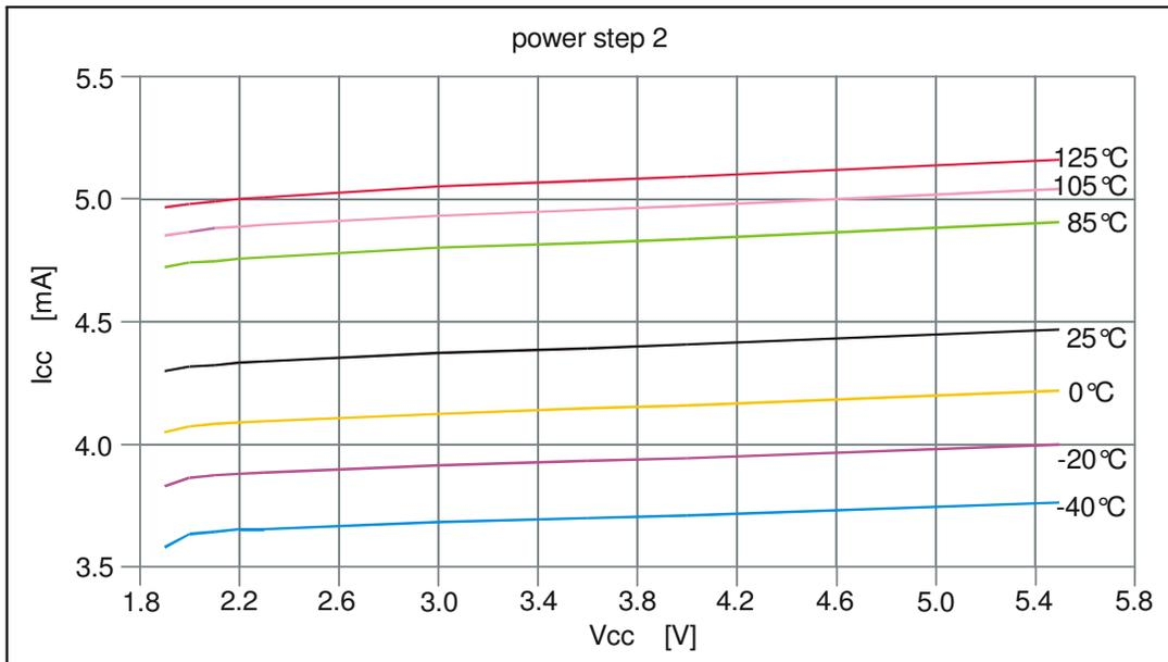
Fig. 9: Supply current in power step 2
