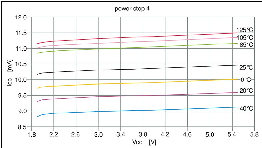
Fig. 11: Supply current in power step 4
