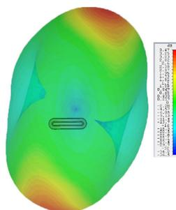
\*3D radiation patterns simulated in CST Microwave Studio on a 600x600mm (2' X2') ground plane with both elements fed together.
