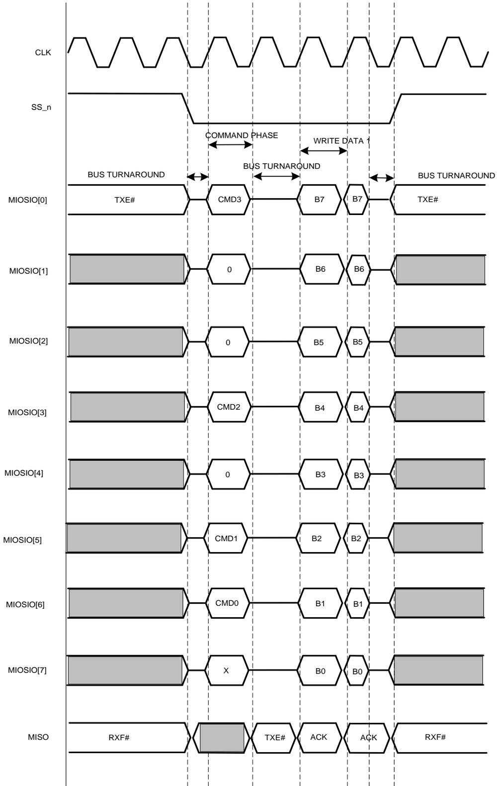
**Figure 8.2 FT1248 8-bit write timing diagram**
