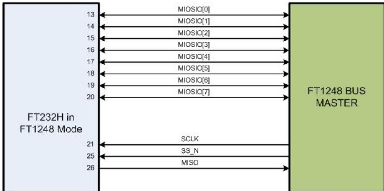
**Figure 8.1 Application Example showing USB to FT1248 host**
