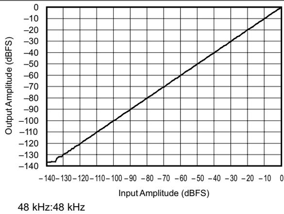
Figure 51. Linearity With  $f_{IN} = 200\text{ Hz}$
