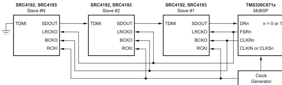
**Figure 74. TDM Interface where all Devices are Slaves**
