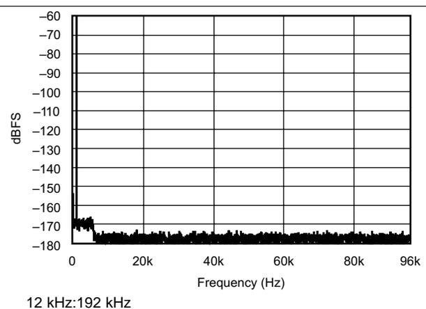
Figure 2. FFT With 1-kHz Input Tone at -60 dBFS
