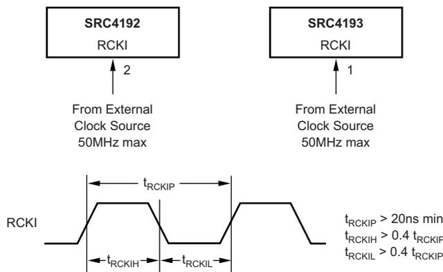
Figure 80. Reference Clock Input Connections and Timing Requirements
