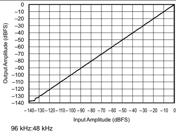
Figure 53. Linearity With  $f_{IN} = 200\text{ Hz}$
