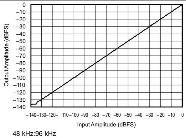
Figure 52. Linearity With  $f_{IN} = 200\text{ Hz}$
