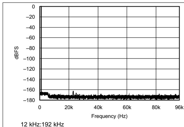
Figure 1. FFT With 1-kHz Input Tone at 0 dBFS
