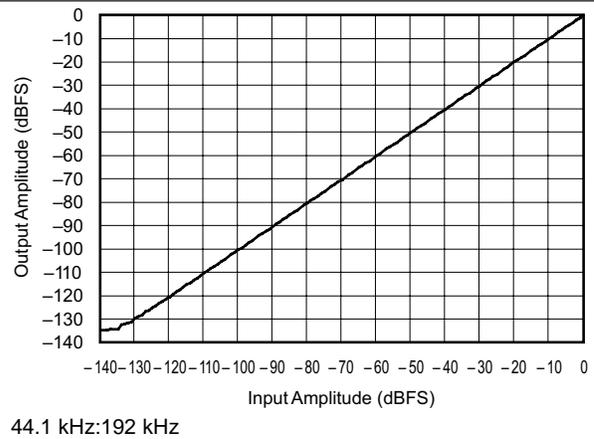
Figure 54. Linearity With  $f_{IN} = 200\text{ Hz}$
