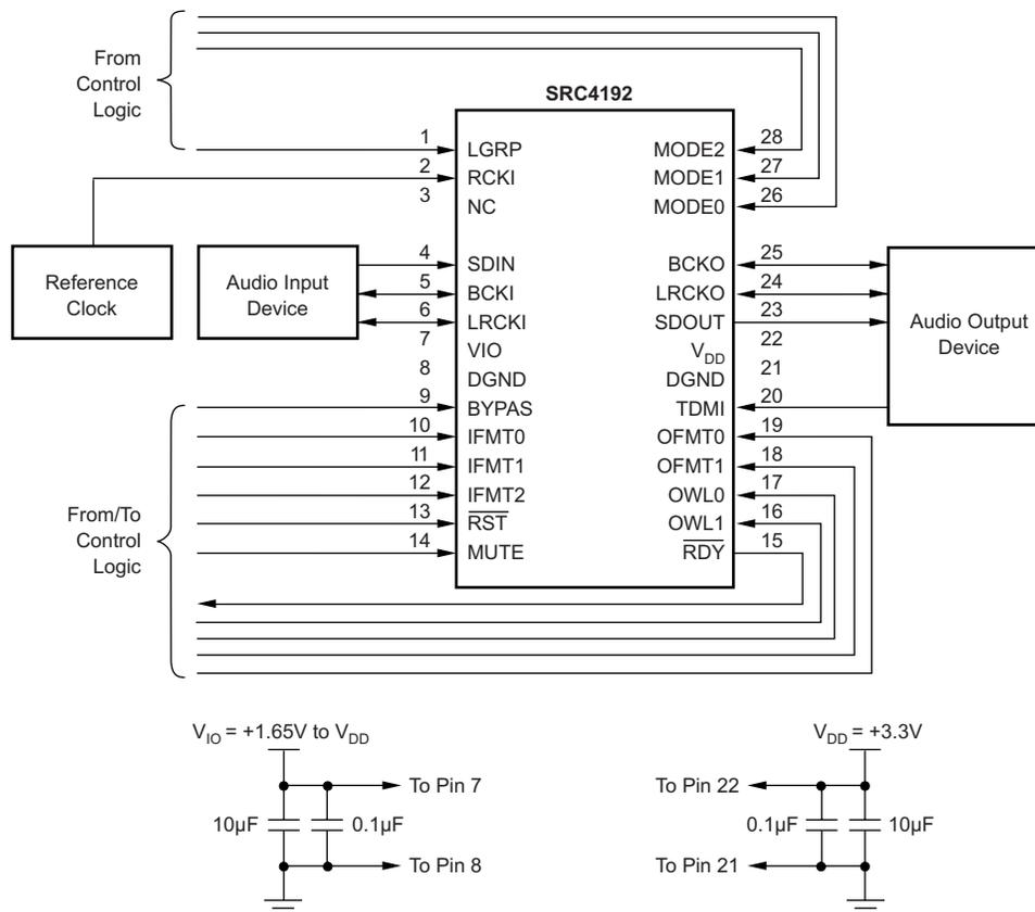
Figure 76. Typical Connection Diagram for the SRC4192
