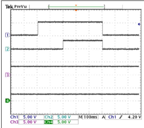
Figure 8. Manual RESET (active-low MR). The active-low MR includes internal debounce circuitry and saves the external active-low MR device. CH1 = active-low MR, CH2 = RESET, CH3 =  $V_{OUT1}$ , CH4 =  $V_{OUT2}$
