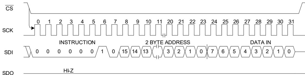
The Adesto RM25C family is capable of a 32-byte write operation.
