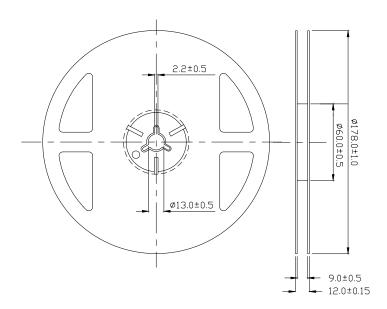
**Note:** The tolerances unless mentioned is  $\pm 0.1$ mm, Angle $\pm 0.5^{\circ}$ , Unit = mm
