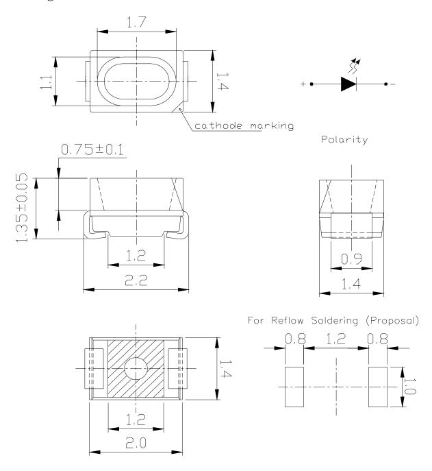
**Notes:** All dimensions are in millimeters. Tolerances unspecified are  $\pm 0.1$ mm.
