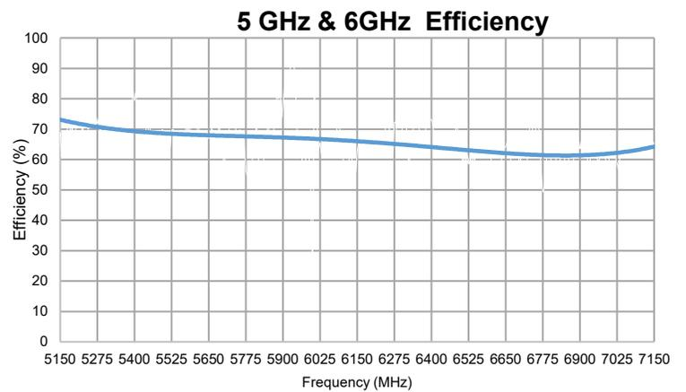
Wi-Fi 2.4 / 5.0 / 6.0 GHz embedded antenna specifications
