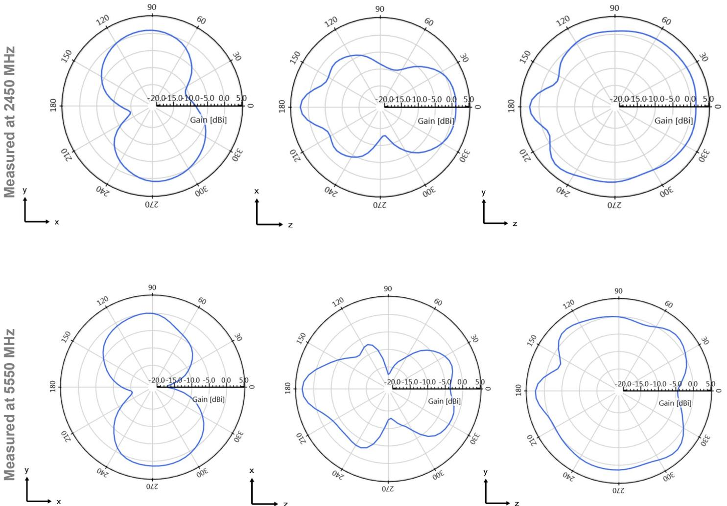
Wi-Fi 2.4 / 5.0 / 6.0 GHz Embedded antenna specifications
