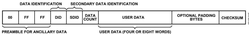
Figure 43. Gemstar and CC Embedded Data Packet (Generic)
