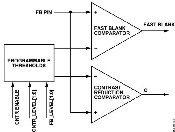
Figure 11. Fast Blank and Contrast Reduction Programmable Threshold
