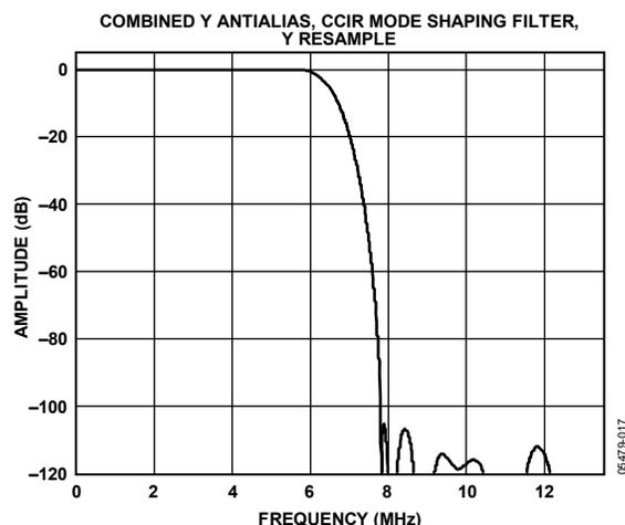
Figure 17. Y SVHS 18 Extra Wideband Filter (CCIR 601 Compliant)
