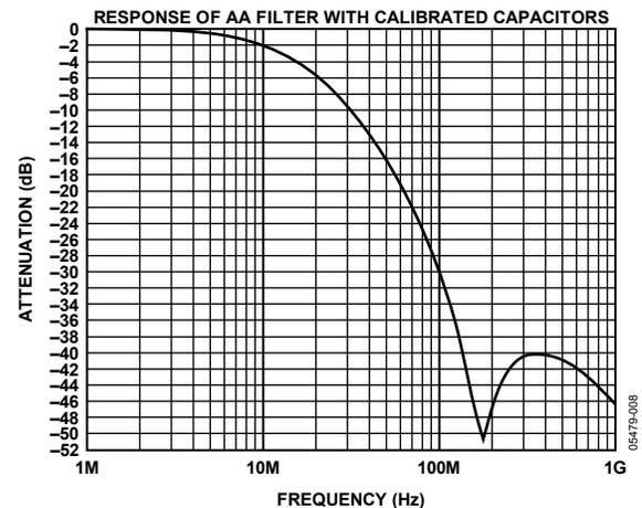
Figure 8. Frequency Response of Internal ADV7184 Antialiasing Filters
