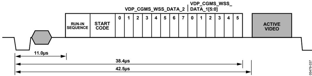
Figure 39. WSS Waveform
