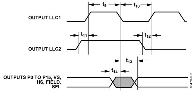
Figure 3. Pixel Port and Control Output Timing
