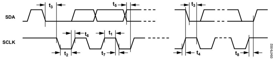
Figure 2. I<sup>2</sup>C Timing
