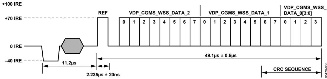
Figure 40. CGMS Waveform
