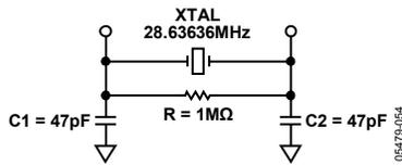
Figure 51. Crystal Circuit
