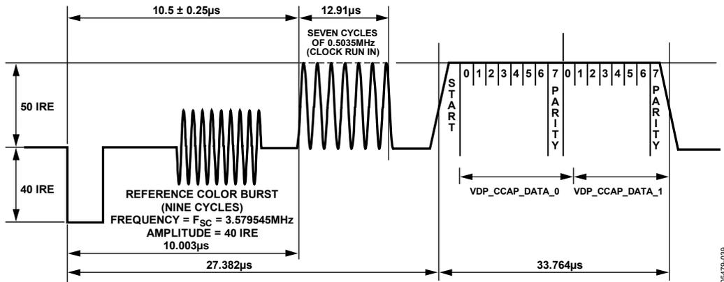
Figure 41. CC Waveform and Decoded Data Correlation
