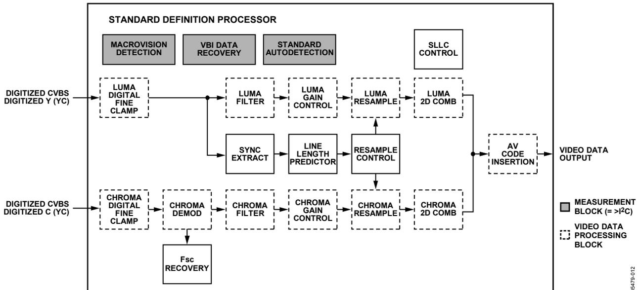
Figure 12. Block Diagram of the Standard Definition Processor
