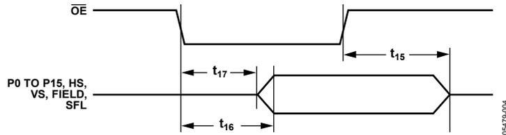
Figure 4.  $\overline{OE}$  Timing
