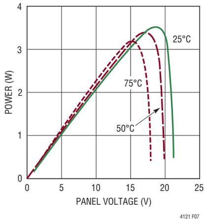
Figure 7. Typical 3W Panel Power vs Voltage
