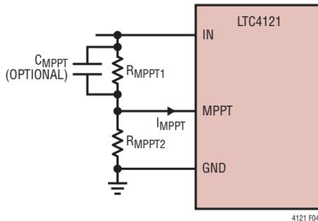
Figure 4. MPPT Resistive Divider
