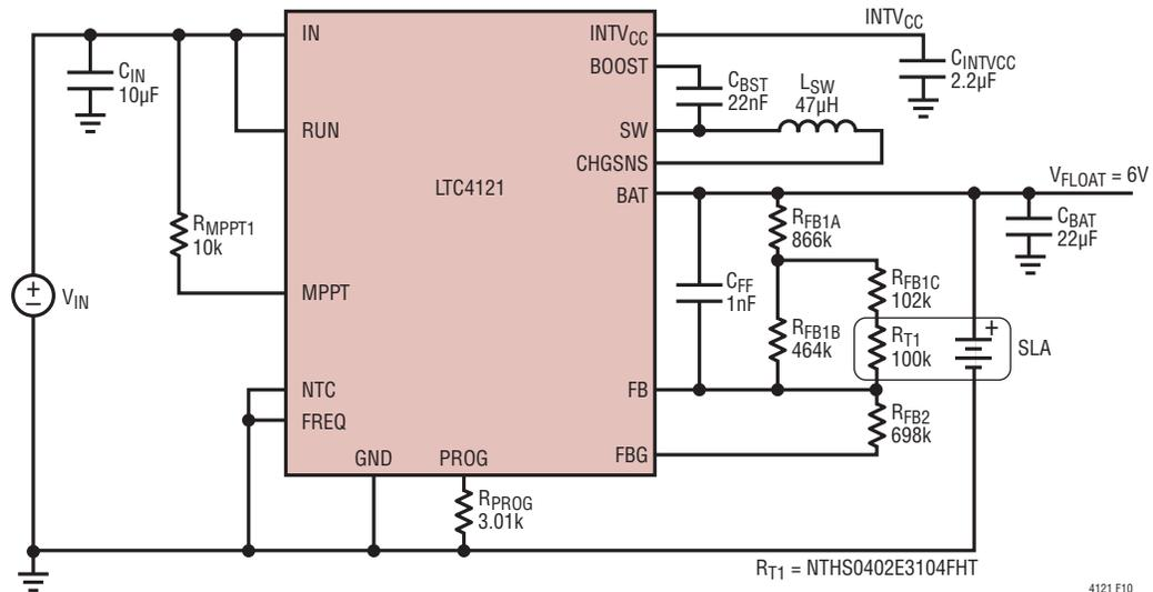
Figure 10. Design Example 3, SLA Charging with LTC4121
