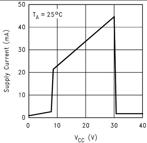
Figure 4. Operating Supply Current vs V<sub>CC</sub>
