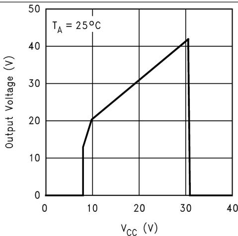
Figure 5. Output Voltage vs V<sub>CC</sub>
