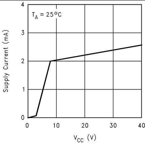
Figure 3. Standby Supply Current vs V<sub>CC</sub>
