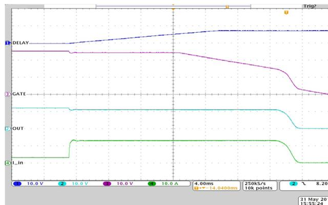
Figure 25. Reverse Overcurrent Protection for Bidirectional Switch
