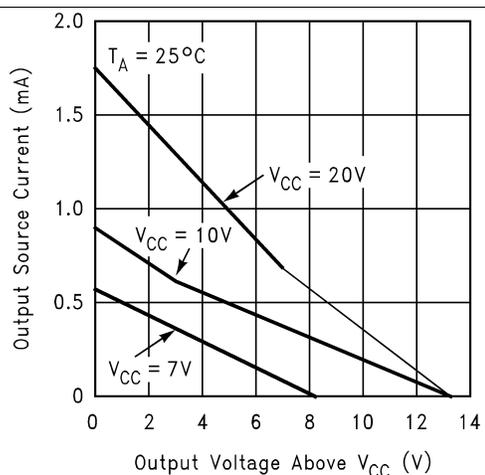
Figure 8. Output Source Current vs Output Voltage
