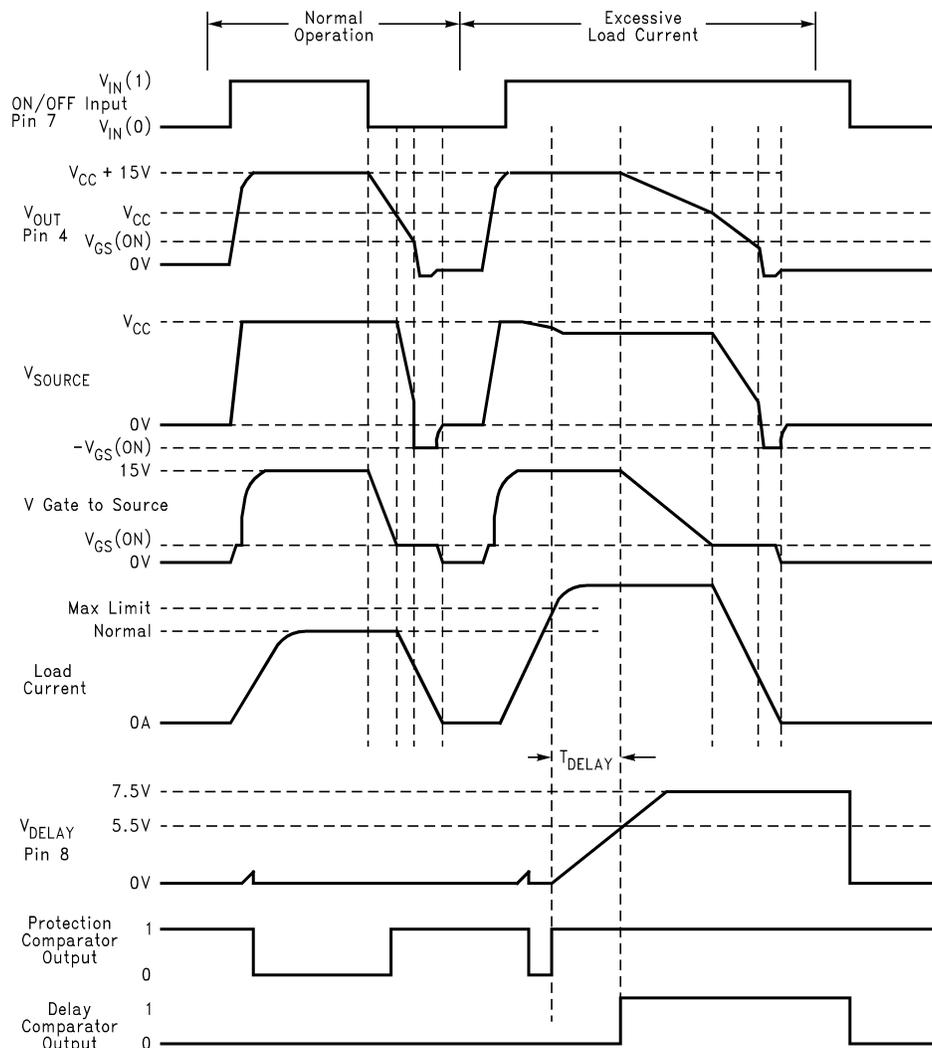
**Figure 1. Typical Operating Waveforms**
