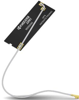
KYOCERA AVX's embedded GNSS Antenna delivers high RF performance and functionality in M2M designs where a more standard GPS patch approach is not possible. This innovative antenna provides compelling advantages for GNSS enabled M2M / IoT applications such as vehicle tracking or asset tracking. Based on a flexible substrate, this GNSS antenna can maintain high efficiency in various device configurations. In addition, the 9000440 antenna can be integrated easily to the end product.
