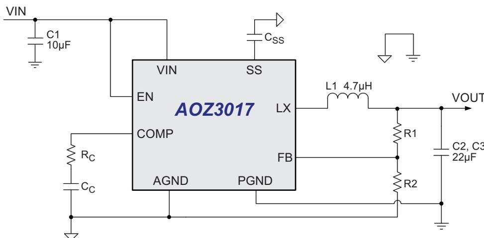
Figure 1. 3.3 V, 4 A Synchronous Buck Regulator,  $F_s = 500$  kHz
