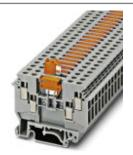
Feed-through terminal block, With test socket screws for insertion of test plugs, Connection type: Screw connection, Cross section: 0.2 mm² - 6 mm², AWG: 24 - 10, Nominal current: 16 A, Nominal voltage: 630 V, Length: 63.5 mm, Width: 6.2 mm, Color: gray, Assembly: NS 35/7,5, NS 35/15, NS 32
