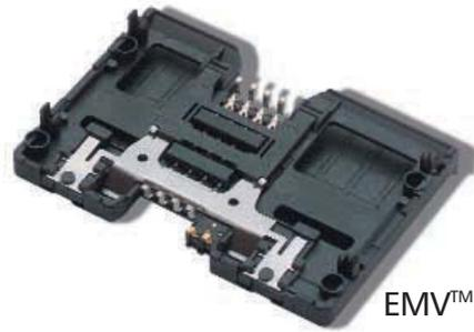
The CCM02 MK II connectors with landing contacts are dedicated for applications where the reader usage is high and the life span of the card is a key consideration. A connector with contacts which land on the card, rather than slide over it, should be specified so as to minimize card wear. The CCM02 has been redesigned to give an even higher performance in a compact, affordable package.
