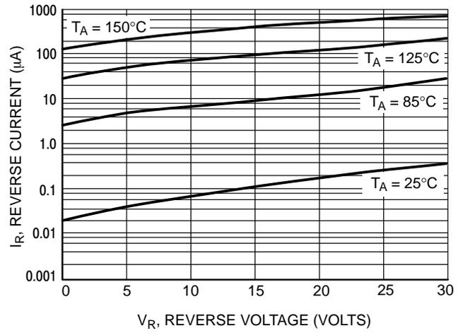
Figure 2. Leakage Current
