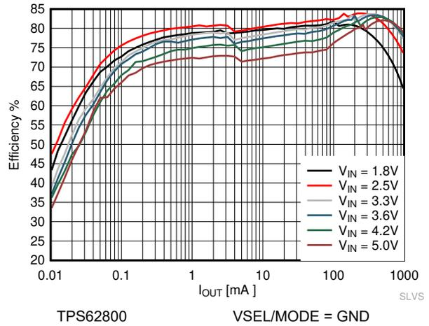
**Figure 9-3. Efficiency Power Save Mode**
