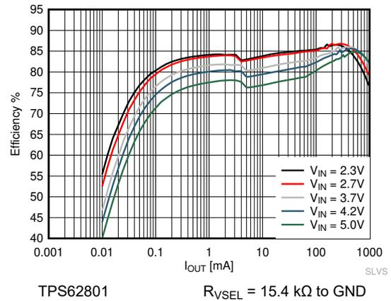
**Figure 9-5. Efficiency Power Save Mode**
