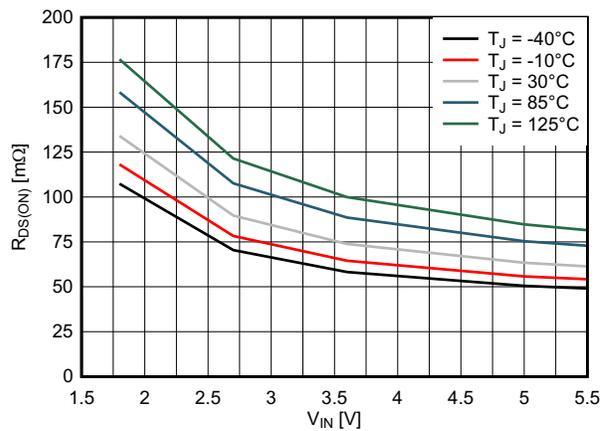
Figure 7-6. Low-Side Switch Drain Source Resistance,  $R_{DS(ON)}$
