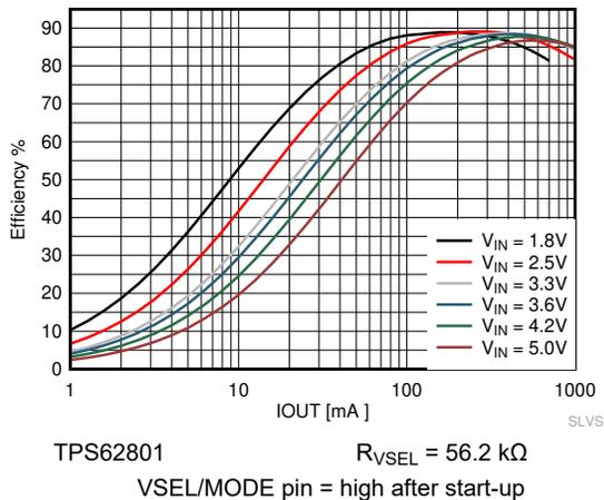
**Figure 9-6. Efficiency Forced PWM Mode**
