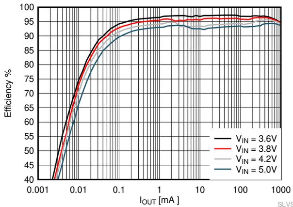
TPS62802  $3.3\text{ V } V_{OUT}$ , VSEL/MODE = 249 k
