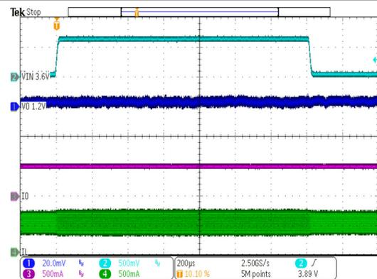
TPS62801  $V_{OUT} = 1.2\text{ V}$   $V_{IN} = 3.6\text{ V to } 4.2\text{ V}$
