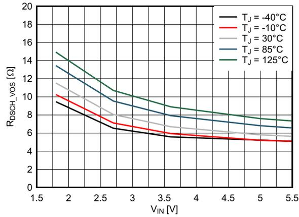
**Figure 7-7. VOS Discharge Switch Drain Source Resistance, R<sub>DSCH\_VOS</sub>**
