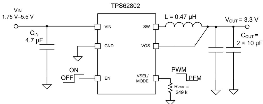
**Figure 9-49. TPS62802 Adjustable 3.3-V  $V_{OUT}$  Application Circuit**
