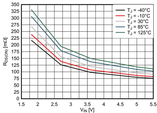
Figure 7-5. High-Side Switch Drain Source Resistance,  $R_{DS(ON)}$
