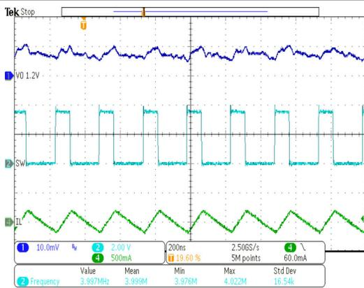
Forced PWM mode  $V_{OUT} = 1.2\text{ V}$   $I_{OUT} = 0\text{ mA}$
