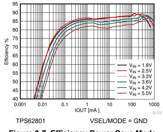
**Figure 9-7. Efficiency Power Save Mode**
