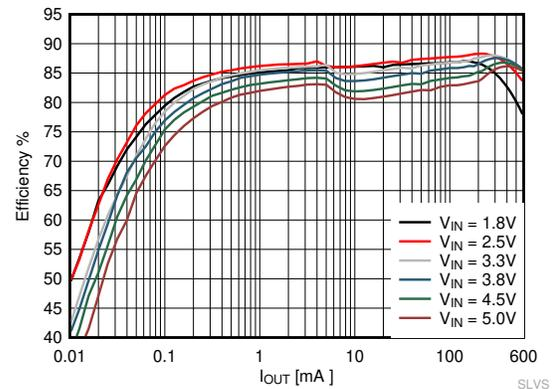
TPS62806  $V_{OUT} = 0.7\text{ V}$ , VSEL/MODE = GND
