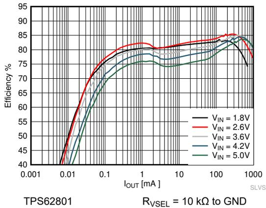
**Figure 9-4. Efficiency Power Save Mode**
