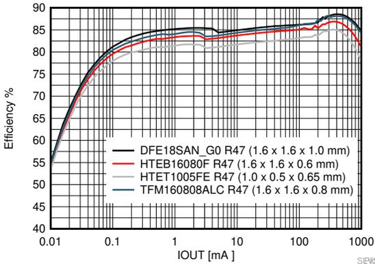
TPS62801 VSEL/MODE = GND,  $V_{OUT} = 1.2\text{ V}$
