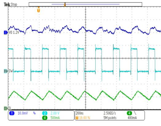
PWM mode  $V_{OUT} = 1.2\text{ V}$   $VSEL/MODE = GND$
