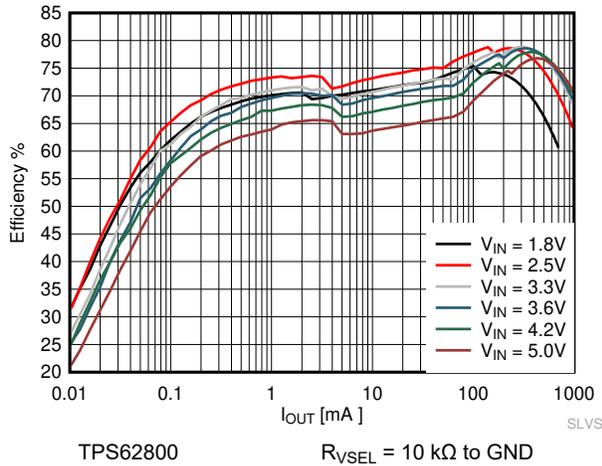
**Figure 9-2. Efficiency Power Save Mode**
