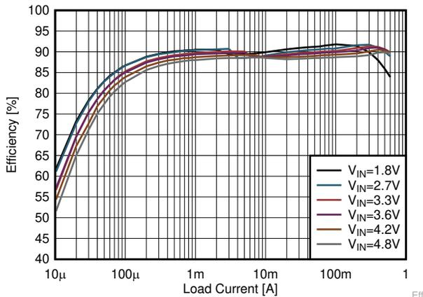
TPS62807  $V_{OUT} = 1.2\text{ V}$ , VSEL/MODE = GND
