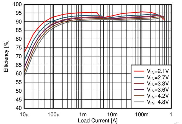
TPS62808  $V_{OUT} = 1.8\text{ V}$ , VSEL/MODE = GND
