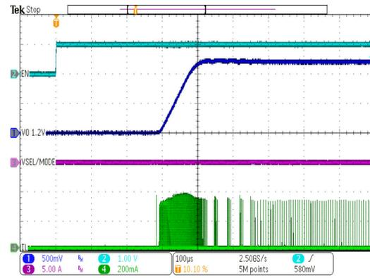
TPS62801       $V_{OUT} = 1.2\text{ V}$        $V_{SEL}/MODE = \text{GND}$
