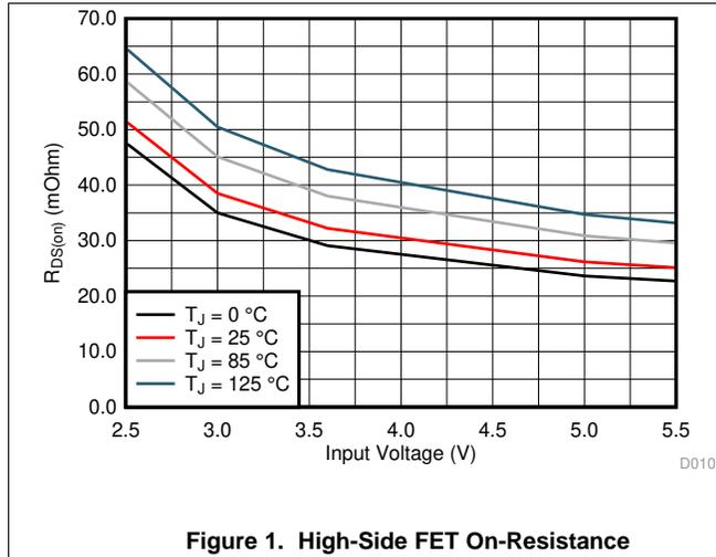
Figure 1. High-Side FET On-Resistance
