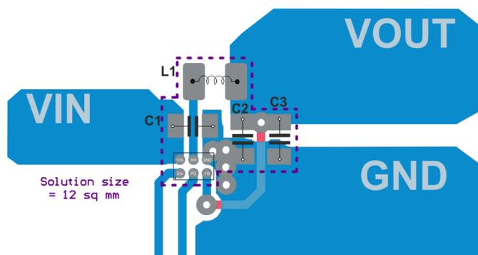
**Figure 15. PCB Layout of Fixed Output Voltage Application**
