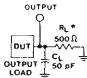
\*FOR AC SERIES ONLY: WHEN  $V_{CC} = 1.5$  V,  $R_L = 1$  k $\Omega$
