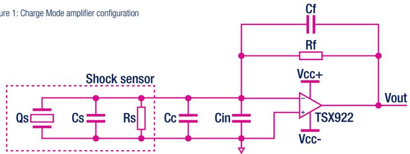
Where  $V_{in}$  is the differential Voltage of the Op amp and  $V_f$  the Voltage in the feedback loop. Thanks to the large gain of the op amp (AVD), and as  $V_{out} = -V_f$  equation 2 can be simplified as equation 3:
