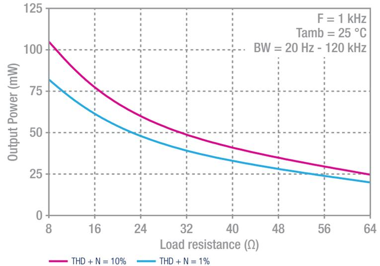
Output power vs. load resistance  $V_{CC} = 5$  V
