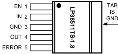
Figure 1. Top View DDPAK/TO-263 5 Pin Package
