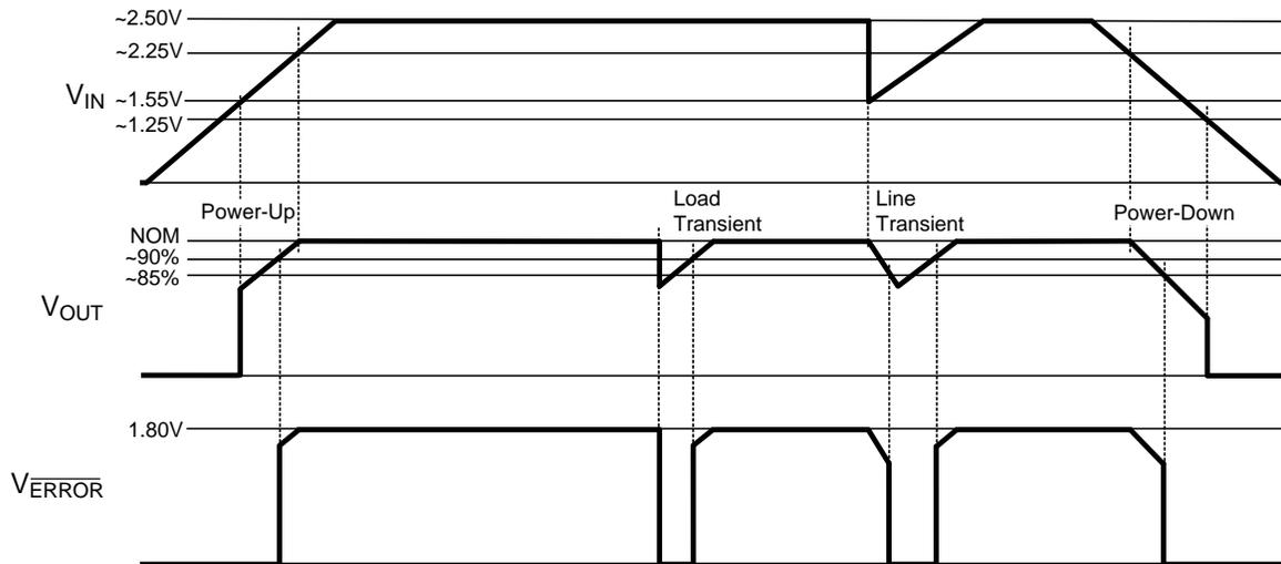
Figure 23.  $\overline{\text{ERROR}}$  Flag Operation, see [Typical Application Circuit](#)
