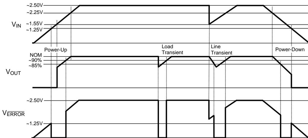
Figure 24.  $\overline{\text{ERROR}}$  Flag Operation, biased from  $V_{IN}$
