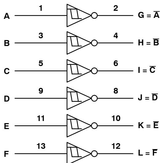
$V_{DD} = \text{Pin}14$
