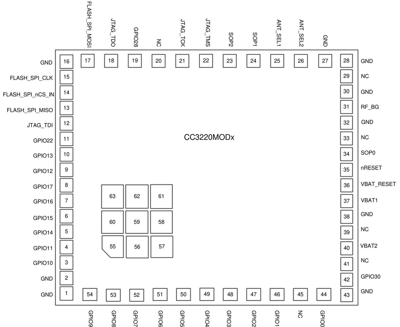
CC3220MODx Pin Diagram Bottom View shows the approximate location of pins on the module. For the actual mechanical diagram, see Section 13.
