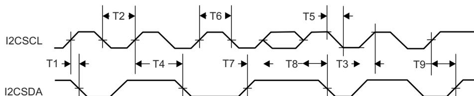
**Figure 8-13. I<sup>2</sup>C Timing Diagram**
