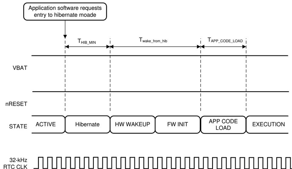
Figure 8-7. Wake Up From Hibernate Timing Diagram
