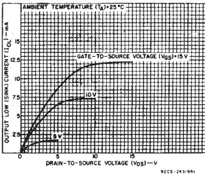
Fig. 6 - Minimum output low (sink) current characteristics.
