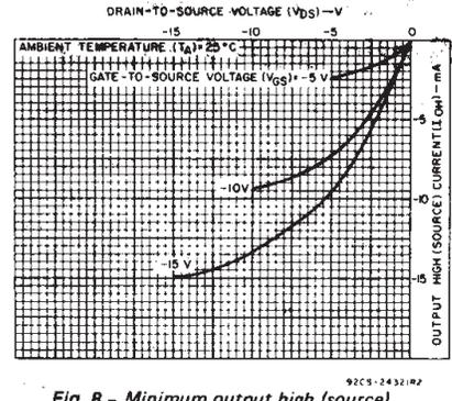
Fig. 8 - Minimum output high (source) current characteristics.
