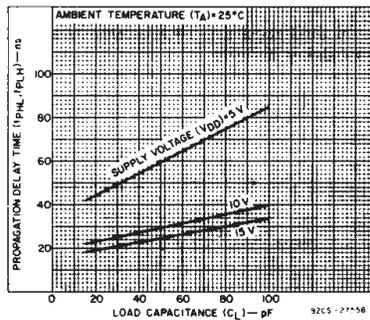
Fig. 10 - Typical propagation delay time vs. load capacitance.
