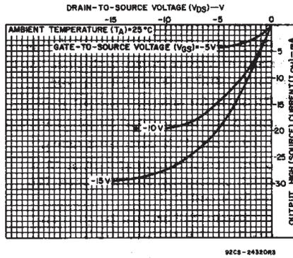
Fig. 7 - Typical output high (source) current characteristics.
