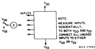
Fig. 14 - Input leakage current test circuit.
