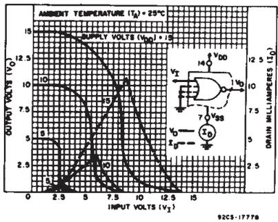
Fig. 3 - Typical current & voltage transfer characteristics.
