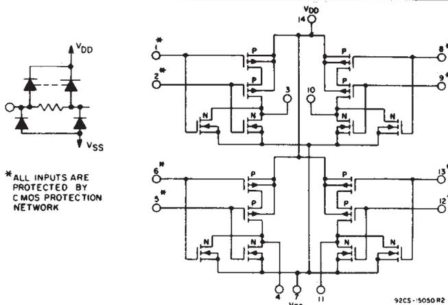
Fig. 4 - Schematic diagram for type CD4001UB.
