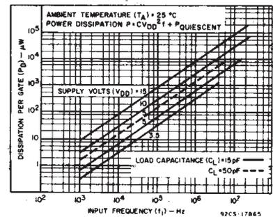
Fig. 11 - Typical power dissipation vs. frequency.
