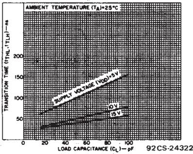
Fig. 9 - Typical transition time vs. load capacitance.
