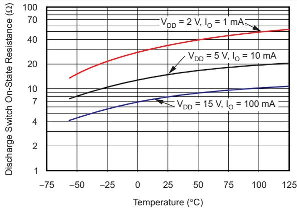
**Figure 1. Discharge Switch On-State Resistance vs Free-Air Temperature**
