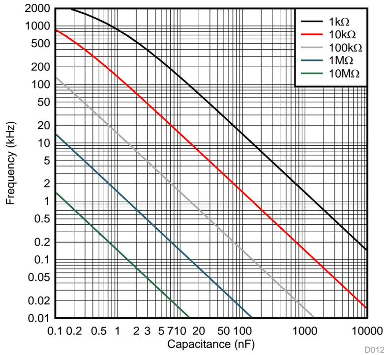
Figure 15. Free-Running Frequency vs Timing Capacitance
