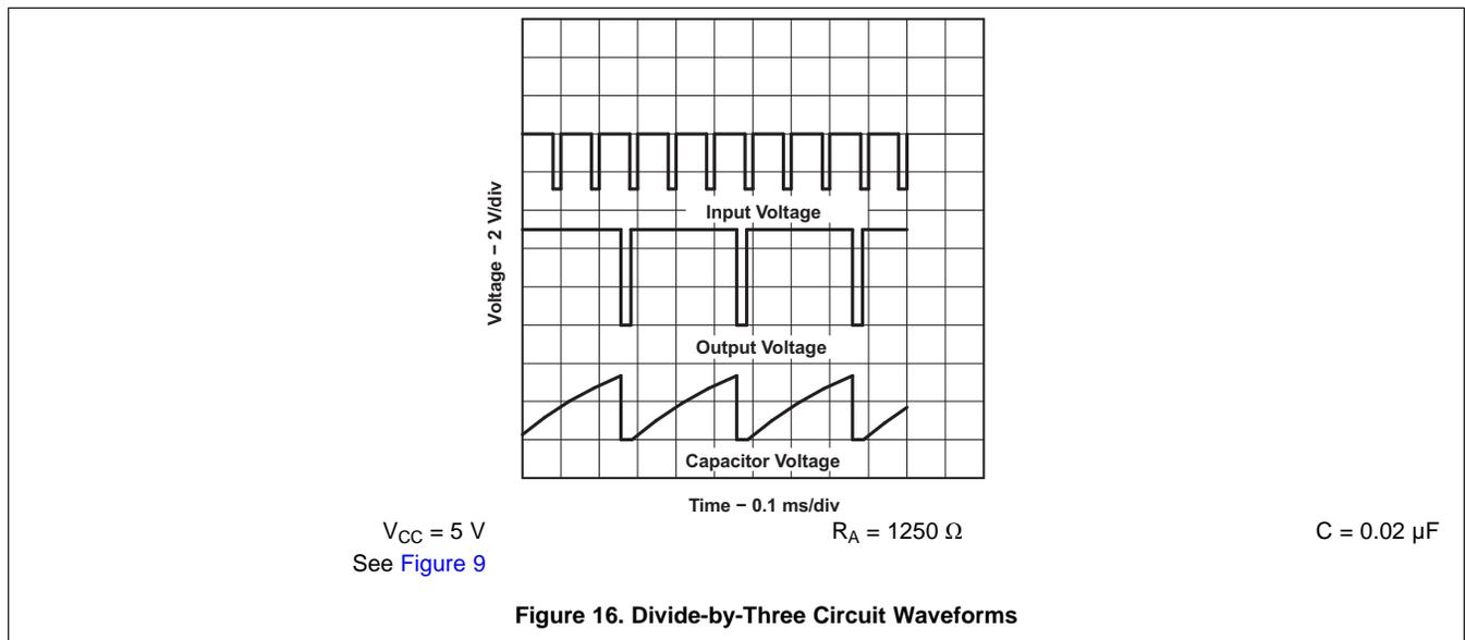
Figure 16. Divide-by-Three Circuit Waveforms
