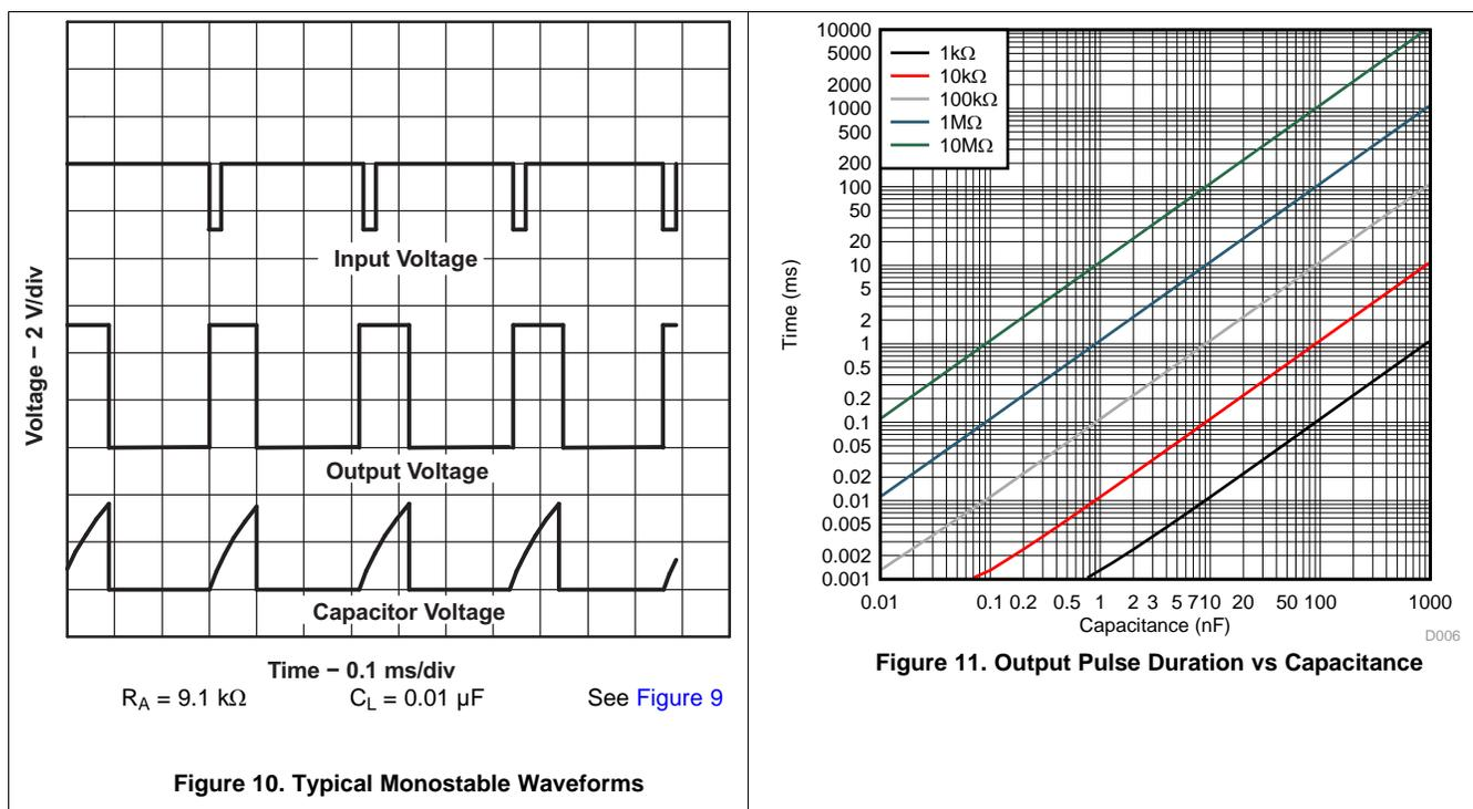
Figure 10. Typical Monostable Waveforms
