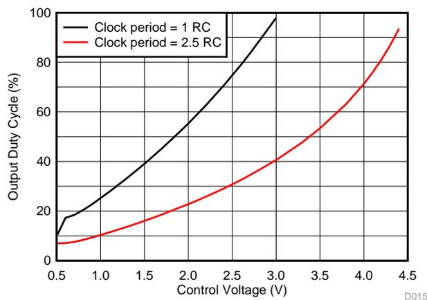
**Figure 21. Pulse-Width-Modulation vs Control Voltage**
