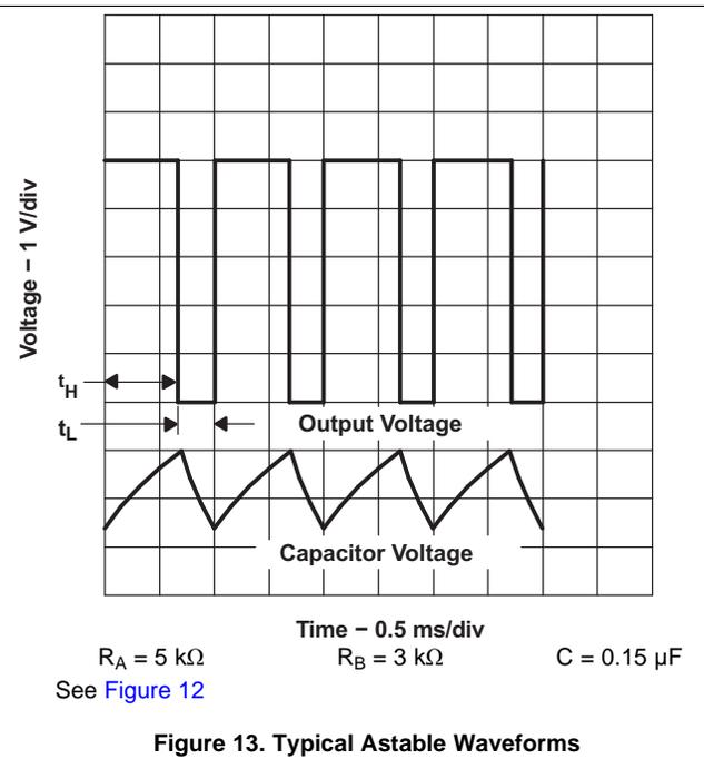
Figure 13 shows typical waveforms generated during astable operation. The output high-level duration  $t_H$  and low-level duration  $t_L$  for frequencies below 100 kHz can be calculated as follows:
