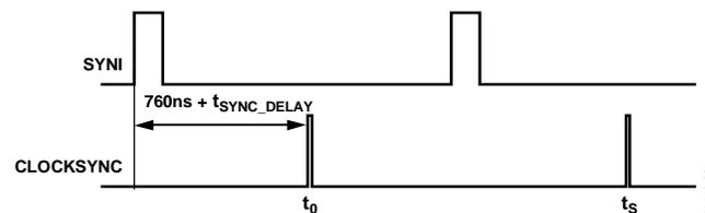
Figure 65. Synchronization Timing
