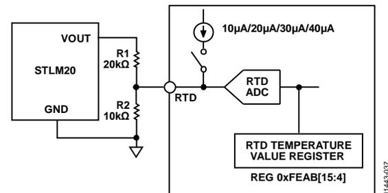
Figure 35. Temperature Sensing by an Analog Temperature Sensor
