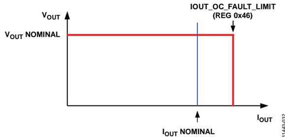
Figure 31. Constant Current Mode ( $V_{OUT}$  vs.  $I_{OUT}$ )
