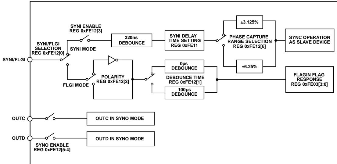
Figure 18. Synchronization Configuration
