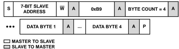
Figure 60. Write Four Bytes to Page 9
