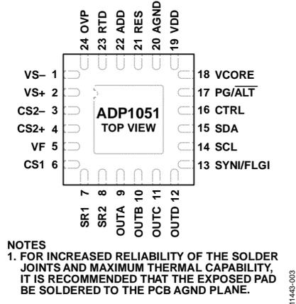
Figure 3. Pin Configuration
