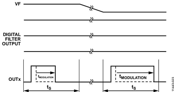
Figure 23. Closed-Loop Input Voltage Feedforward Changes Modulation Values
