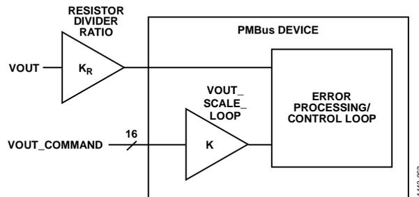
Figure 63. Conceptual View of the VOUT\_SCALE\_LOOP Command
