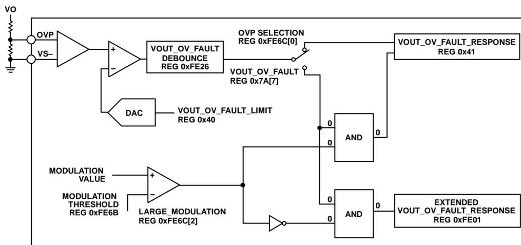
Figure 38. V<sub>OUT</sub> Overvoltage Protection Circuit Implementation
