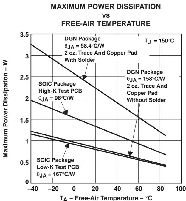
NOTE A: Results are with no air flow and PCB size = 3"× 3"
