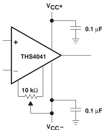
Figure 66. Offset Nulling Schematic
