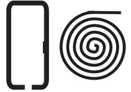
Figure 33: Loop or Trace Antenna
