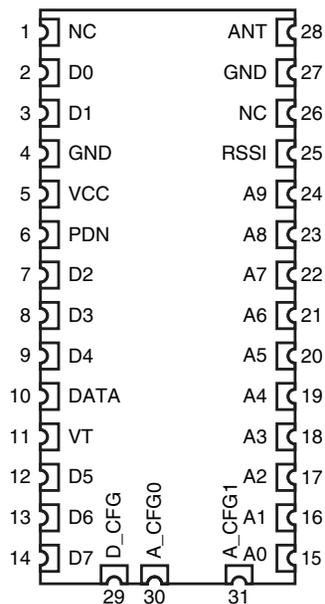
Figure 9: KH3 Series Receiver Pinout (Top View)
