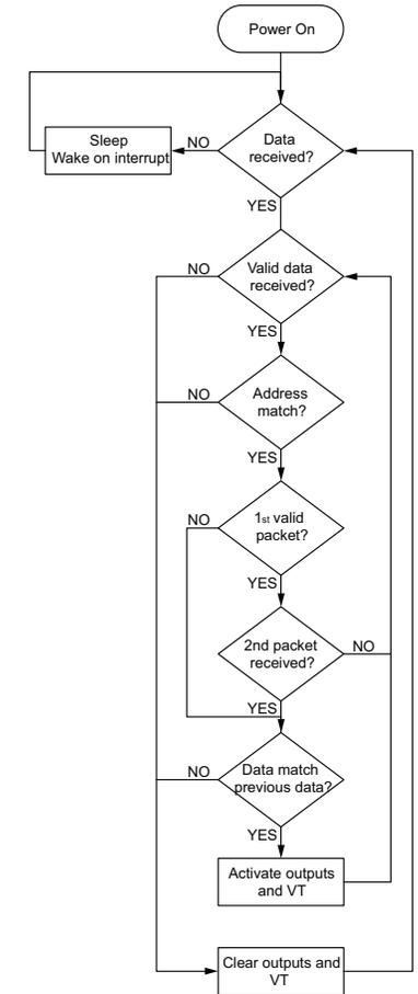
Figure 12: KH3 Series Receiver / Decoder Flowchart
