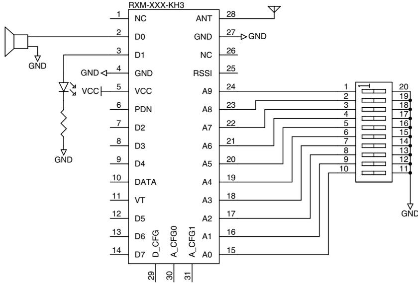
Figure 17: KH3 Series Receiver Typical Application Circuit
