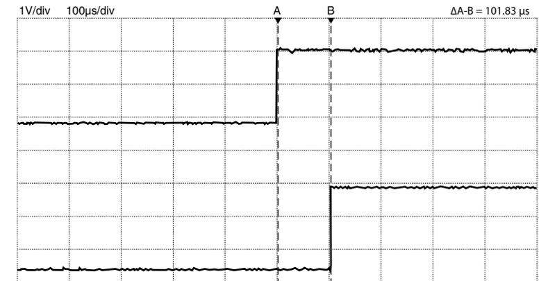
Figure 6: KH3 Series Receiver Turn-On Time from PDN
