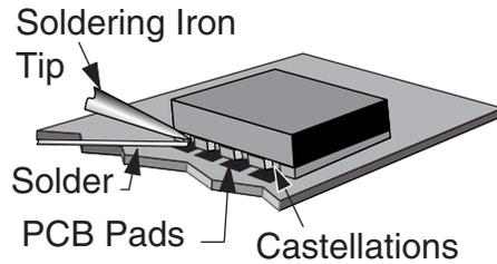
Figure 24: Soldering Technique
