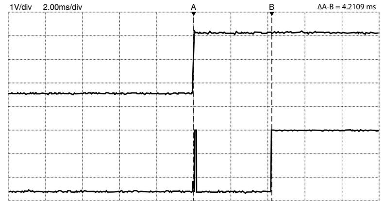
Figure 5: KH3 Series Receiver Turn-On Time from  $V_{CC}$
