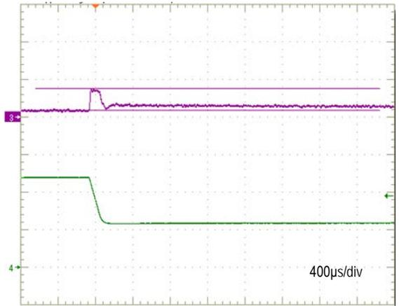
Start-up ( $V_{in}=48V$ ,  $V_{out}=5V$ ,  $I_{out}=12A$ ,  $T_a=+25^{\circ}C$ )
