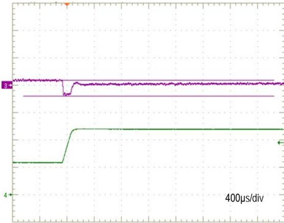
Transient Response ( $V_{in}=48V$ ,  $I_{out}=12A$  to  $6A$ ,  $T_a=+25^{\circ}C$ )
