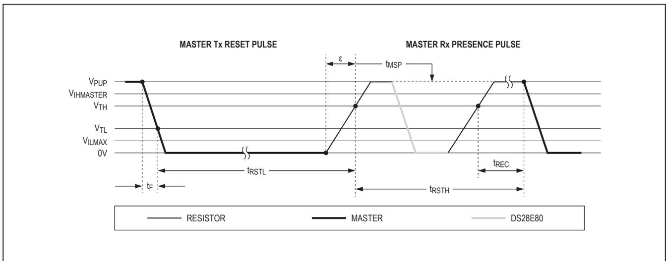
Figure 9. Reset/Presence pulse
