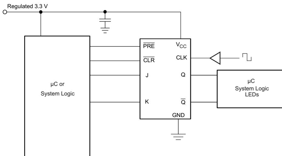
**Figure 5. Typical Application Schematic**
