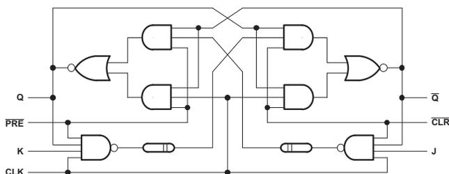
Figure 4. Logic Diagram, Each Flip-Flop (Positive Logic)
