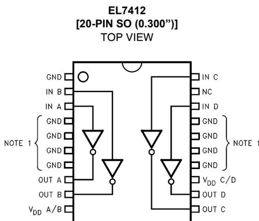
Note 1: Pins 4-7 and 14-17 are electrically connected.
