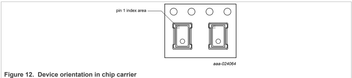
Figure 12. Device orientation in chip carrier
