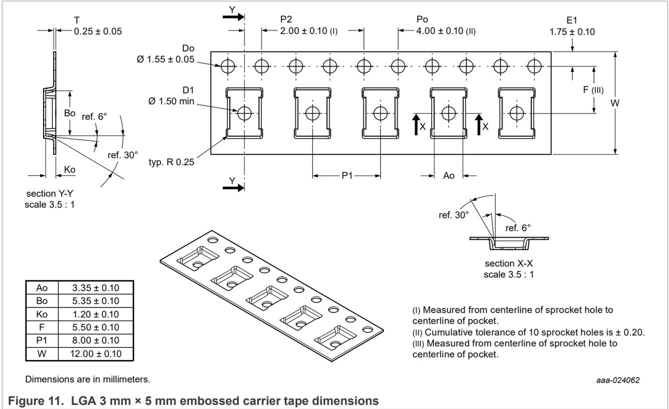
Figure 11. LGA 3 mm × 5 mm embossed carrier tape dimensions
