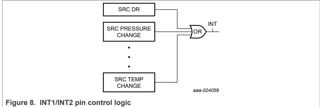
Figure 8. INT1/INT2 pin control logic
