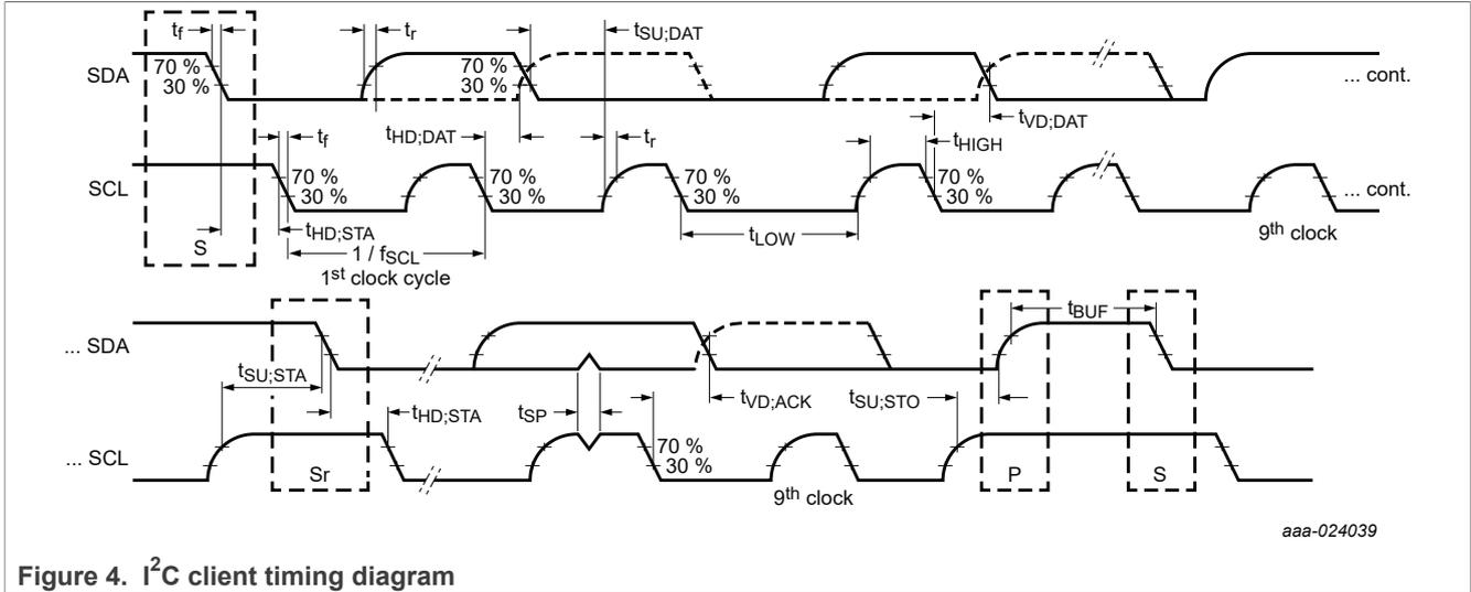
Figure 4. I<sup>2</sup>C client timing diagram
