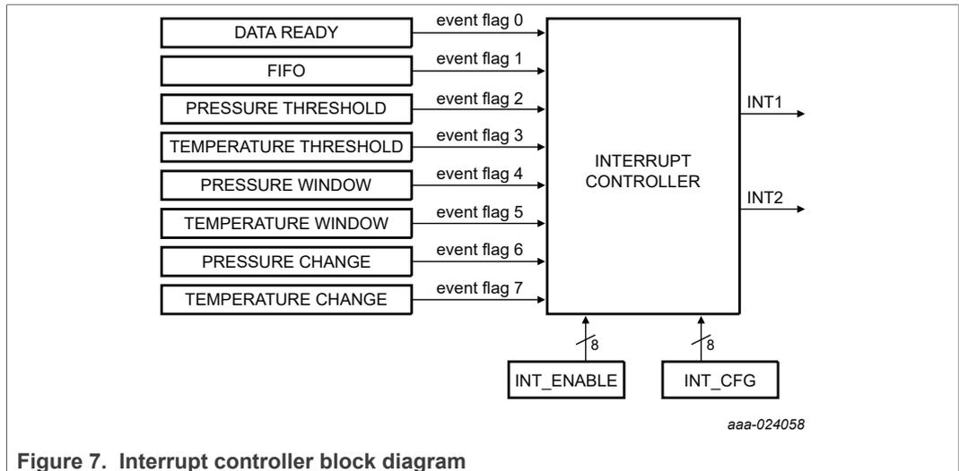
Figure 7. Interrupt controller block diagram
