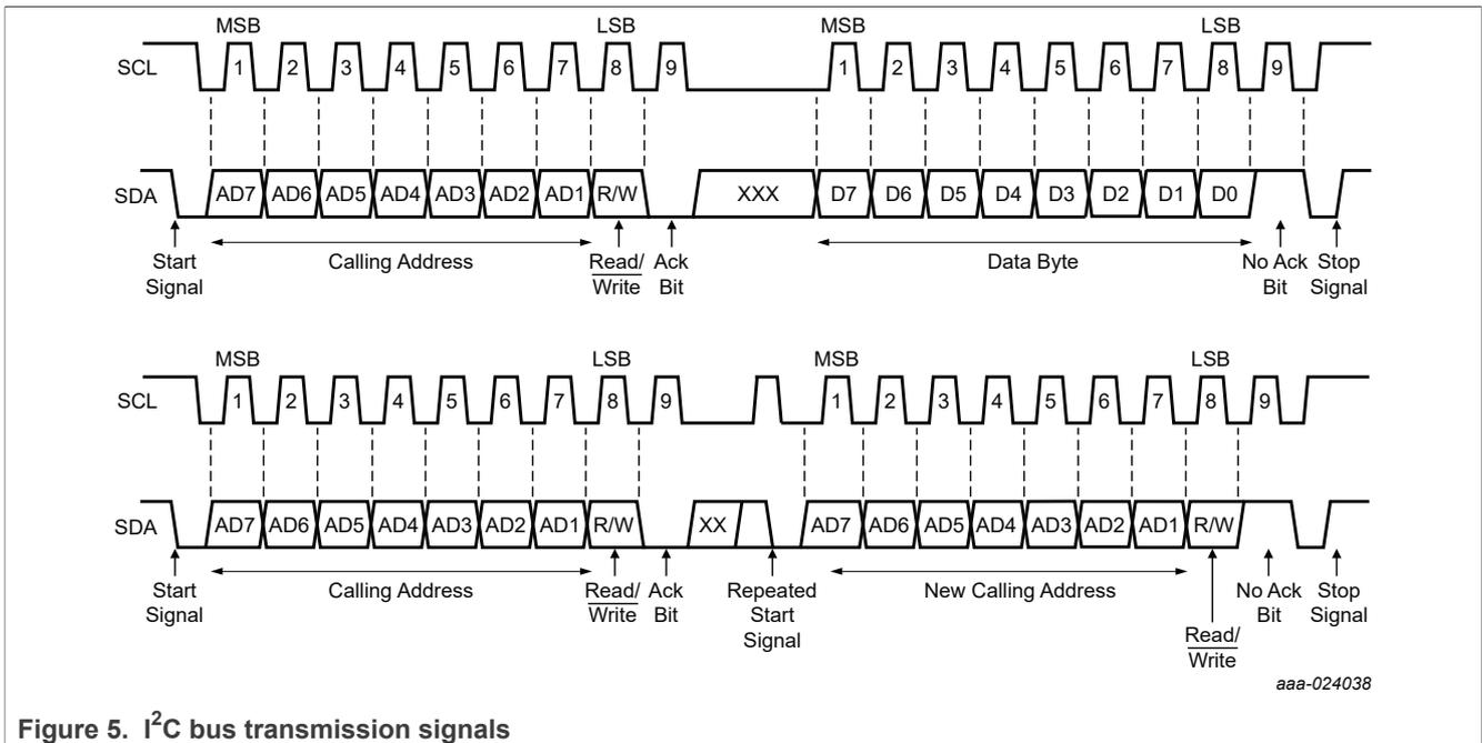
Figure 5. I<sup>2</sup>C bus transmission signals
