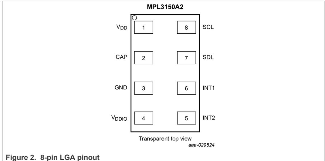
Figure 2. 8-pin LGA pinout
