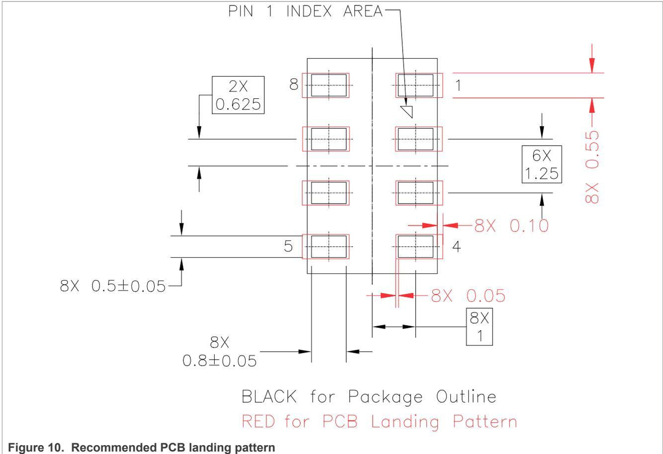
Figure 10. Recommended PCB landing pattern
