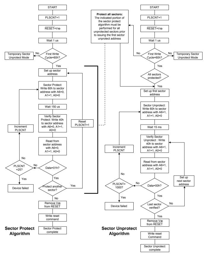
Figure 2. In-System Sector Protect/Unprotect Algorithms
