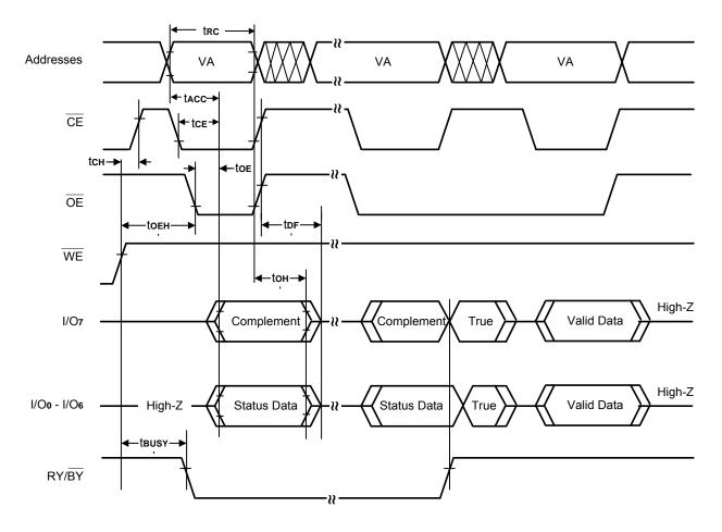
Note: VA = Valid Address. Illustation shows first status cycle after command sequence, last status read cycle, and array data read cycle.
