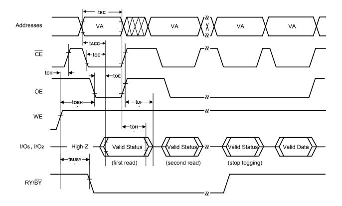
Note: VA = Valid Address; not required for I/O<sub>6</sub>. Illustration shows first two status cycle after command sequence, last status read cycle, and array data read cycle.
