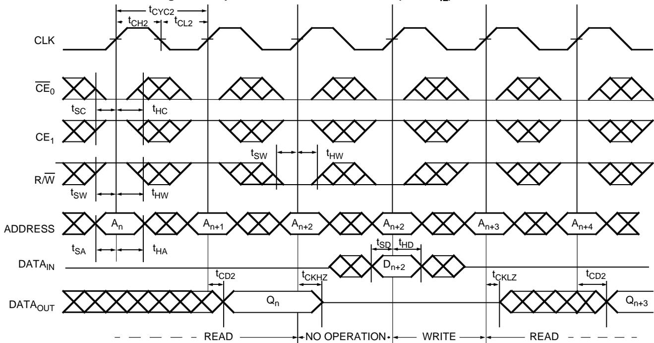
Figure 7. Pipelined Read-to-Write-to-Read (OE Controlled) [15, 16, 17, 18]
