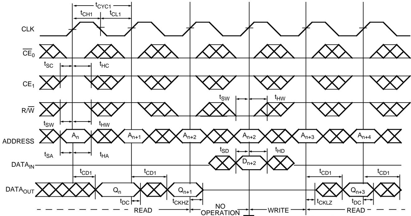
Figure 9. Flow-through Read-to-Write-to-Read (OE Controlled)<sup>[19, 20, 21, 22, 23]</sup>
