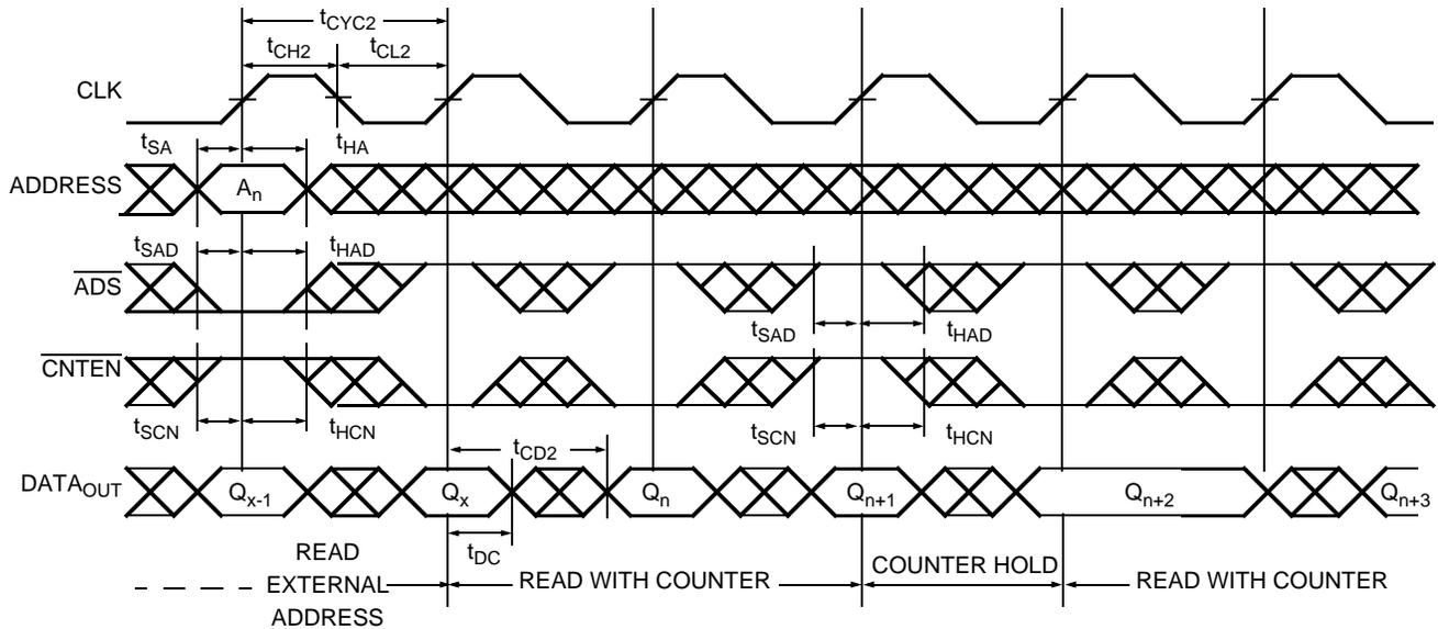
Figure 11. Flow-through Read with Address Counter Advance<sup>[24]</sup>
