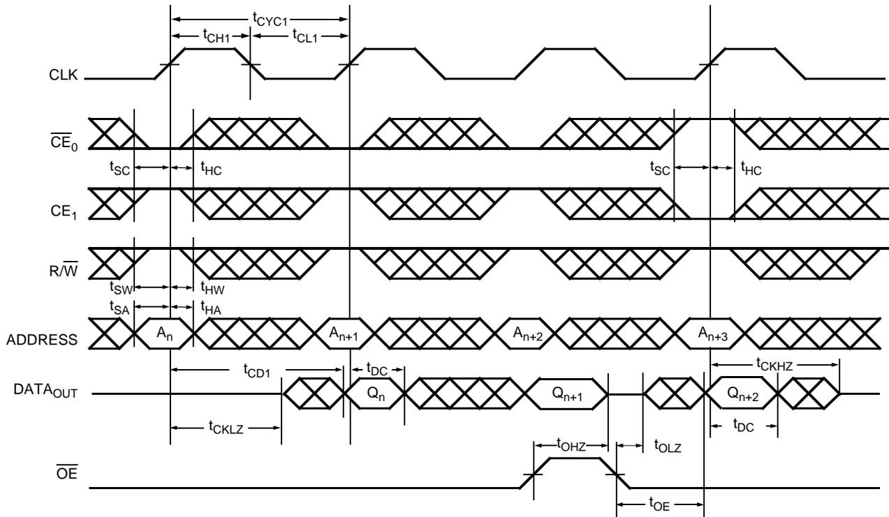
Figure 3. Read Cycle for Pipelined Operation ( $\overline{\text{FT/PIPE}} = V_{\text{IH}}$ )<sup>[5, 6, 7, 8]</sup>
