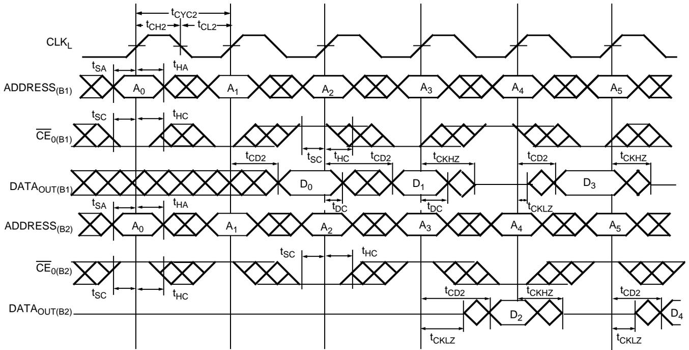
Figure 5. Left Port Write to Flow-through Right Port Read<sup>[11, 12, 13, 14]</sup>
