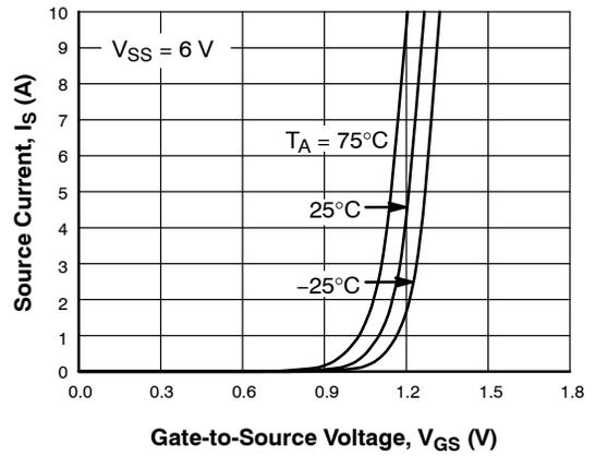
Figure 3. Transfer Characteristics
