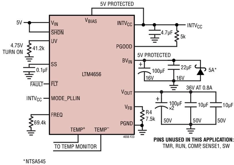
Figure 23. 5V Input to 36V<sub>OUT</sub> at 0.8A Design
