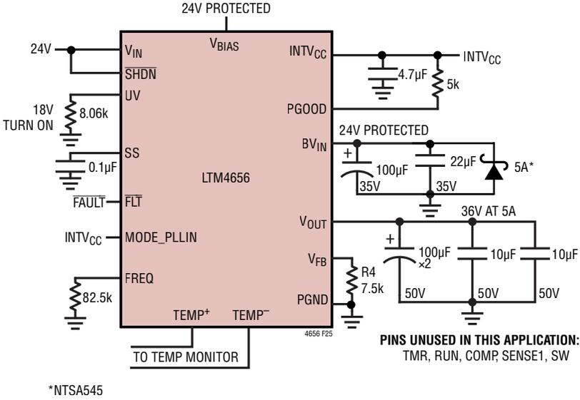
Figure 25. 24V Input to 36V<sub>OUT</sub> at 5A Design
