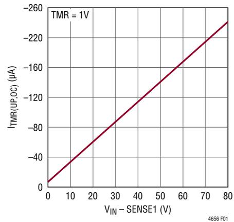
Figure 1. Overcurrent TMR Current vs  $V_{IN} - \text{SENSE1}$  Voltage
