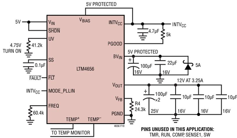
Figure 19. 5V Input to 12V<sub>OUT</sub> at 3.25A Design
