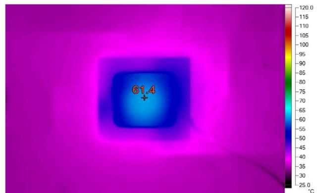
**Figure 7. 12V<sub>IN</sub> to 24V<sub>OUT</sub> at 4A (96W), 200LFM Air Flow Thermal Plot**
