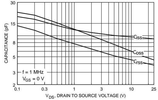
Figure 8. Capacitance Characteristics.
