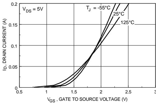
Figure 5. Transfer Characteristics.
