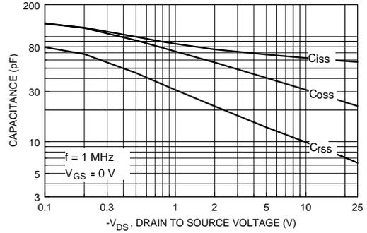
Figure 18. Capacitance Characteristics.
