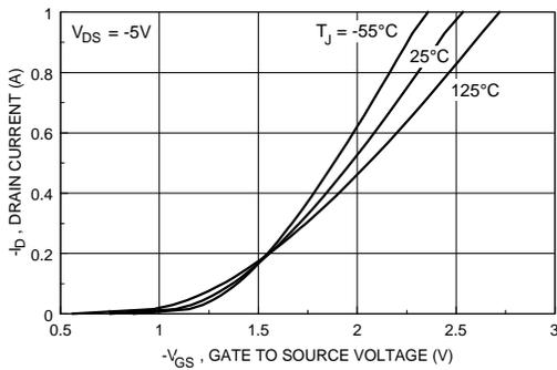
Figure 15. Transfer Characteristics.
