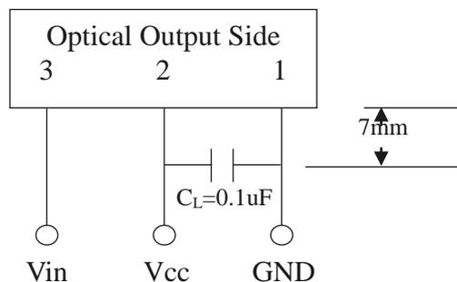
PCB Layout for Electrical Circuit
