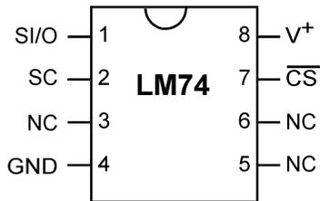
**Figure 2. SOIC – Top View**
