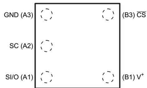
**Figure 3. 5-Bump DSBGA – Top View**
