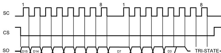
Figure 15. b) Reading Continuous Conversion - Two Eight-Bit Frames
