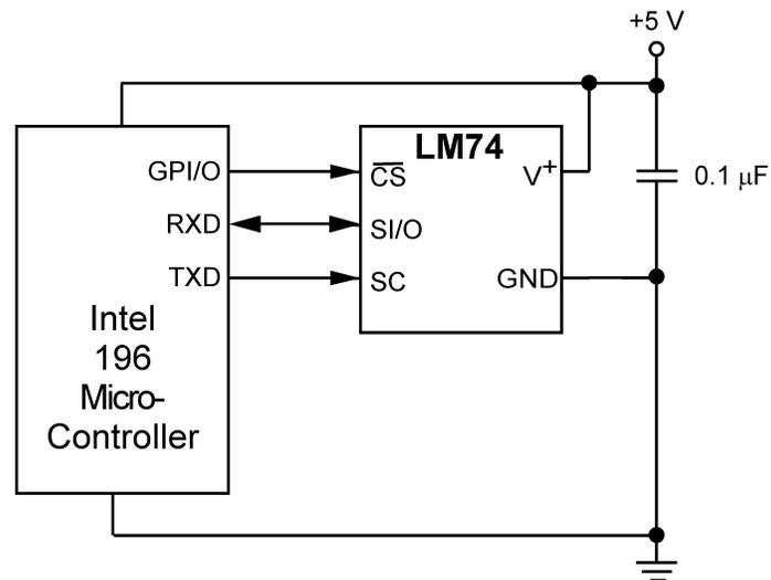
Figure 17. Temperature monitor using Intel 196 processor
