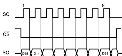
Figure 14. a) Reading Continuous Conversion - Single Eight-Bit Frame
