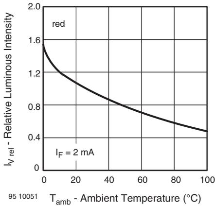
Fig. 4 - Relative Luminous Intensity vs. Ambient Temperature
