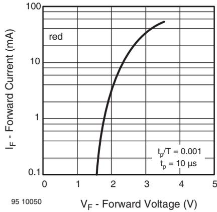
Fig. 3 - Forward Current vs. Forward Voltage
