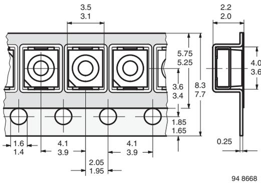
Fig. 8 - Tape Dimensions in mm for PLCC-2
