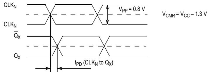
**Figure 4. MC100ES6221 AC Test Reference Measurement Waveform**
