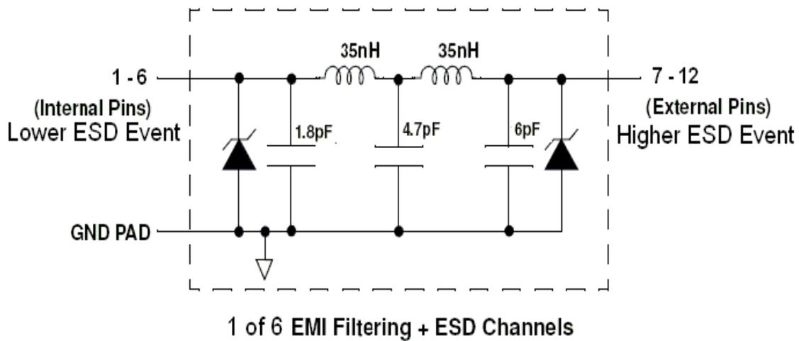
**Figure 1. Electrical Schematic**
