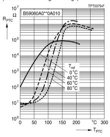
PTC resistance  $R_{\text{PTC}}$  versus PTC temperature  $T_{\text{PTC}}$  (measured at low signal voltage)
