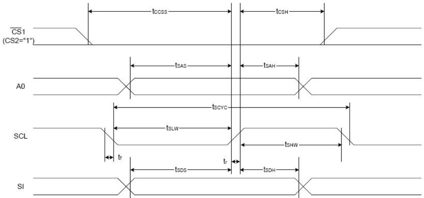
\*1 The input signal rise and fall time ( $t_r$ ,  $t_f$ ) are specified at 15 ns or less.
